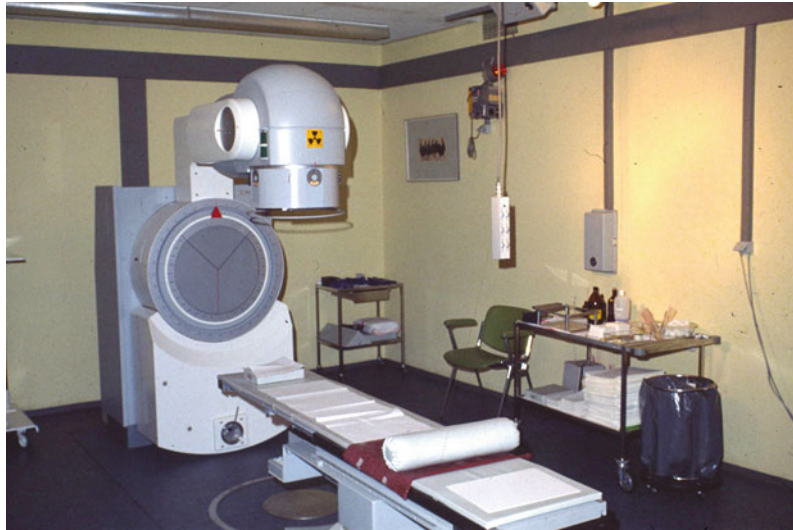
History of Radiation Oncology. Fig. 10 Telecobalt-60 machine with 80 cm source-skin distance manufactured by Philips
