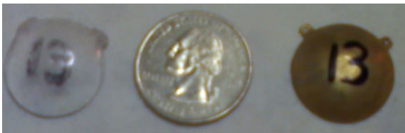
Eye Plaque Physics. Fig. 4 A picture of a round plaque and its associated plastic dummy. The coin is shown for size reference
