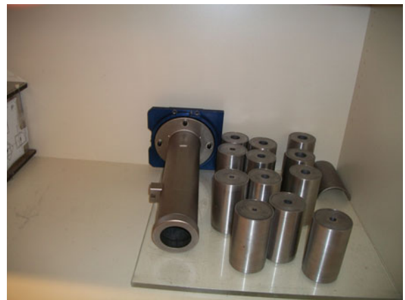
Stereotactic Radiosurgery – Cranial. Fig. 2 Picture of the linac attachment cone and multiple collimators used for cone-based stereotactic radiosurgery
