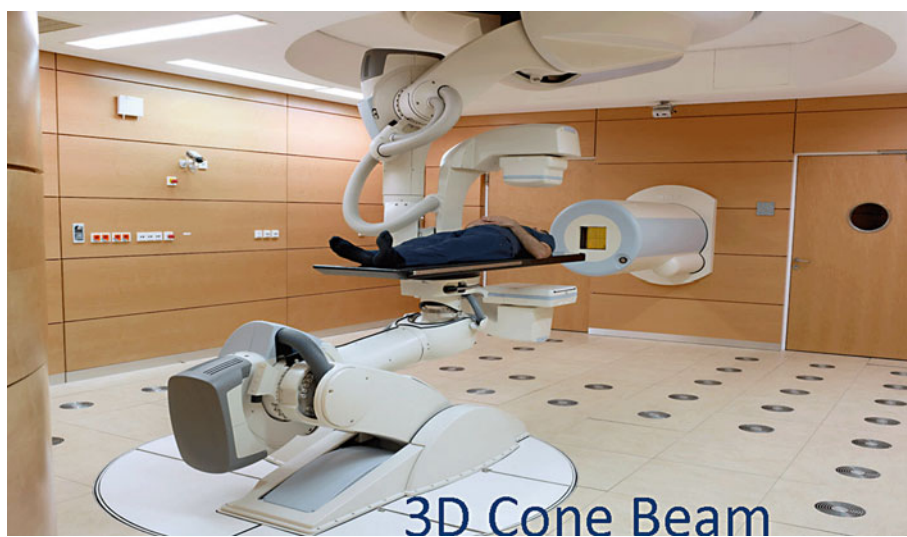
Image-Guided Radiation Therapy (IGRT): kV Imaging. Fig. 4 Robotic controlled CBCT system, HIT proton facility, Heidelberg, Germany
