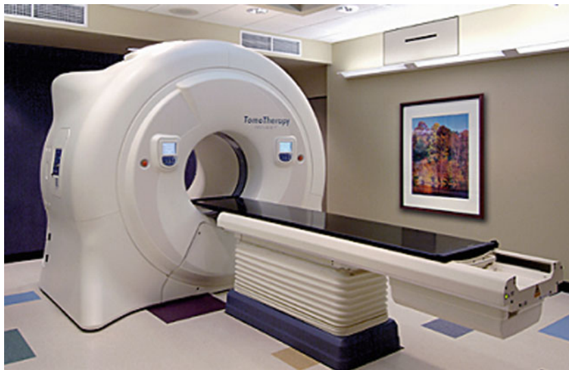
Image-Guided Radiation Therapy (IGRT): TomoTherapy. Fig. 1 The Hi-ART helical tomotherapy CT-guided IMRT system
