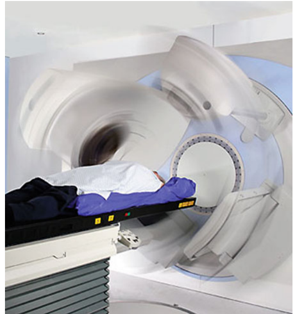
Image-Guided Radiation Therapy (IGRT): kV Imaging. Fig. 3 Linac-integrated kV CBCT system, Elekta
