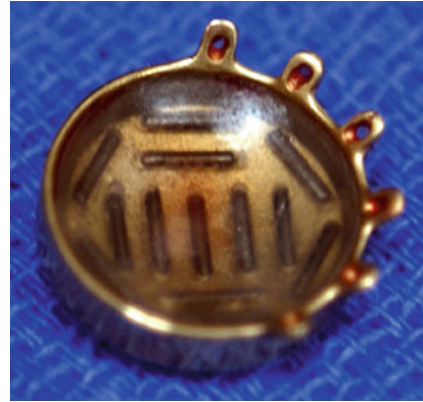
Eye and Orbit. Fig. 2 COMS plaque with I-125 seeds and inset
