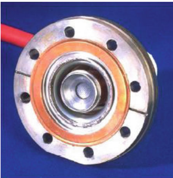
Linear Accelerators (LINAC). Fig. 6 Removable electron triode gun from a high-energy linac, Varian Clinac-18 (From Podgorsak 2005)
