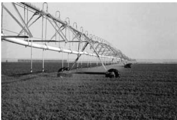
Fig. 71.1 A centre pivot irrigation system.
