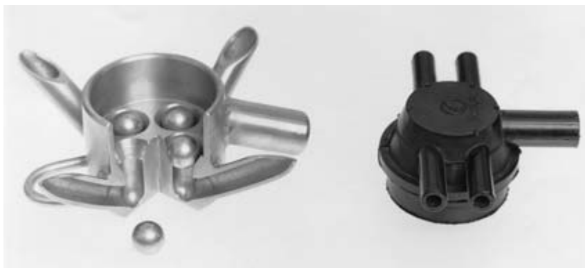
Fig. 26.9 Ball claw cluster. Photo courtesy of Institute of Animal Health (IAH), Compton.
