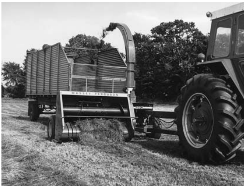
Fig. 4.13 Silage making with a precision chop forage harvester.
