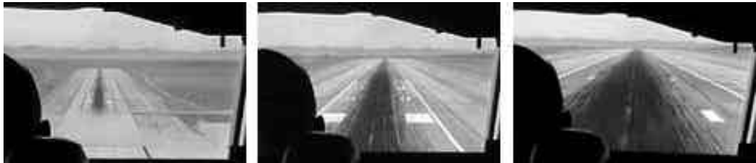
Figure 17. Pilot views of MD-11 performing a PCA Instrument Landing System-coupled approach and landing.
