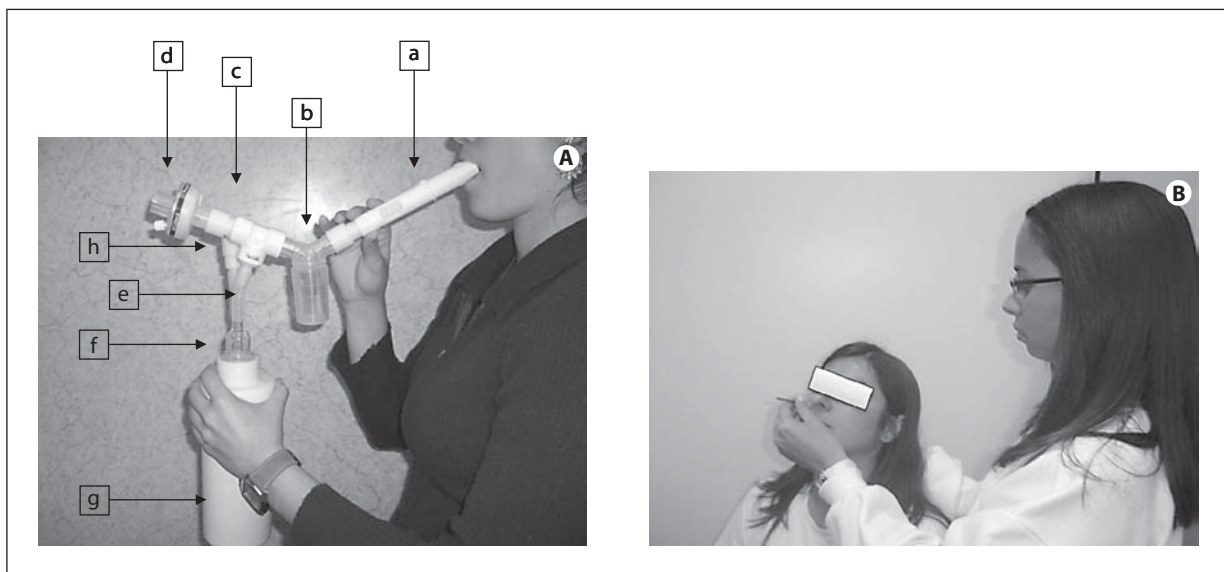
Fig. 3. The exhaled breath condensator modified apparatus (A): (a) buccal, (b) saliva collector, (c) T-piece with unidirectional valve, (d) filter (humid vent filter compact S, Louis Gibeck AB, Upplands Väsby, Sweden), (e) EBC tube connector, (f) EBC tube collector, (g) condenser reservoir, and (h) expiratory unidirectional valve. This apparatus was developed by Dr. Paulo Hilário Nascimento Saldiva, Dr. Naomi Kondo Nakagawa, Simão Bacht, and Dr. Idágene Cestari, and built by Bioengineering Division of Heart Institute (InCor) University of São Paulo Medical School; STT test (B).
