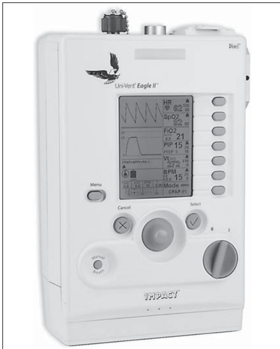
Fig. 1. A sophisticated portable ventilator capable of ventilating critically ill patients. This device has an internal air source (compressor) and a suite of monitoring and alarms allowing it to be used in a number of situations.
