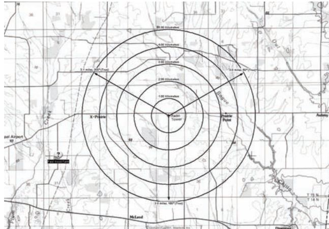
Figure 4. Coverage map indicating the non-line-of-sight coverage area advertised by Motorola. 5 km is typical non-line-of-sight coverage while we actually were getting 9+ km under non-line-of-sight conditions
