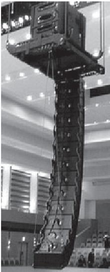
Figure 10.9 Example of a line array speaker, suspended in a concert hall. Top box shows a sub-woofer, lower than 80 Hz.
