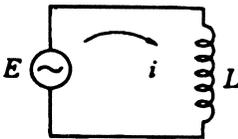
Figure 11.2 Electric circuit with an inductance.
