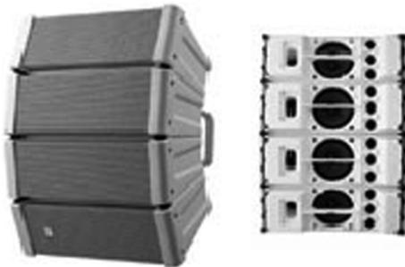
*Figure 10.11* Compact array speaker. Woofer 12 cm, cone  $\times$  4 and dome tweeter  $\times$  12. Crossover: 4 kHz. Directivity: H:  $100^\circ \times V$ : variable =  $15^\circ, 30^\circ, 45^\circ, 60^\circ$ , depending on assembly style. Program input: 450 W/unit. Right side: without front net.
