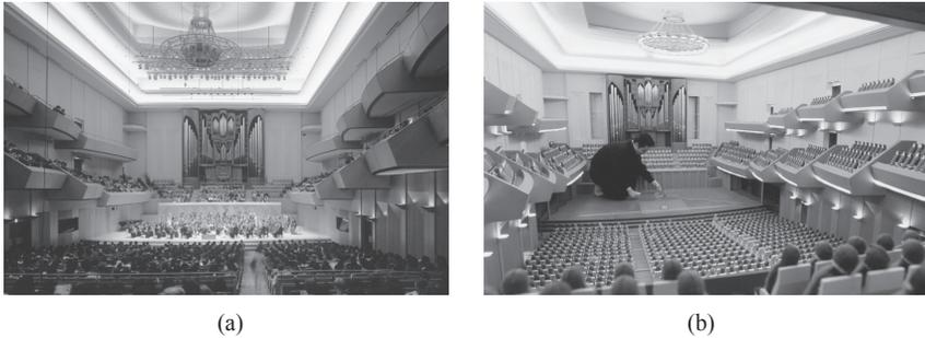
Figure 9.20 The Yokohama Minato-Mirai Concert Hall (a), and the experimental 1/10 scale model of the same (b). Reproduced with permission from H. Tachibana (2010).
