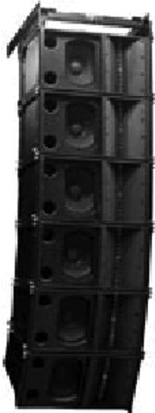
*Figure 10.10* Line array speaker. Woofer 30 cm, cone and horn tweeter. Crossover: 1000 Hz. Directivity: H:  $90^\circ \times V: 5\text{--}15^\circ/\text{unit}$ . Program input: 450 W/unit.
