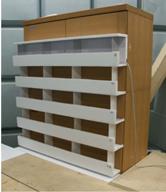
Fig. 7.40 Chest used for scale-model experiment ( 1 \times 0.45 \times 1.35 \text{ m}^3 )
