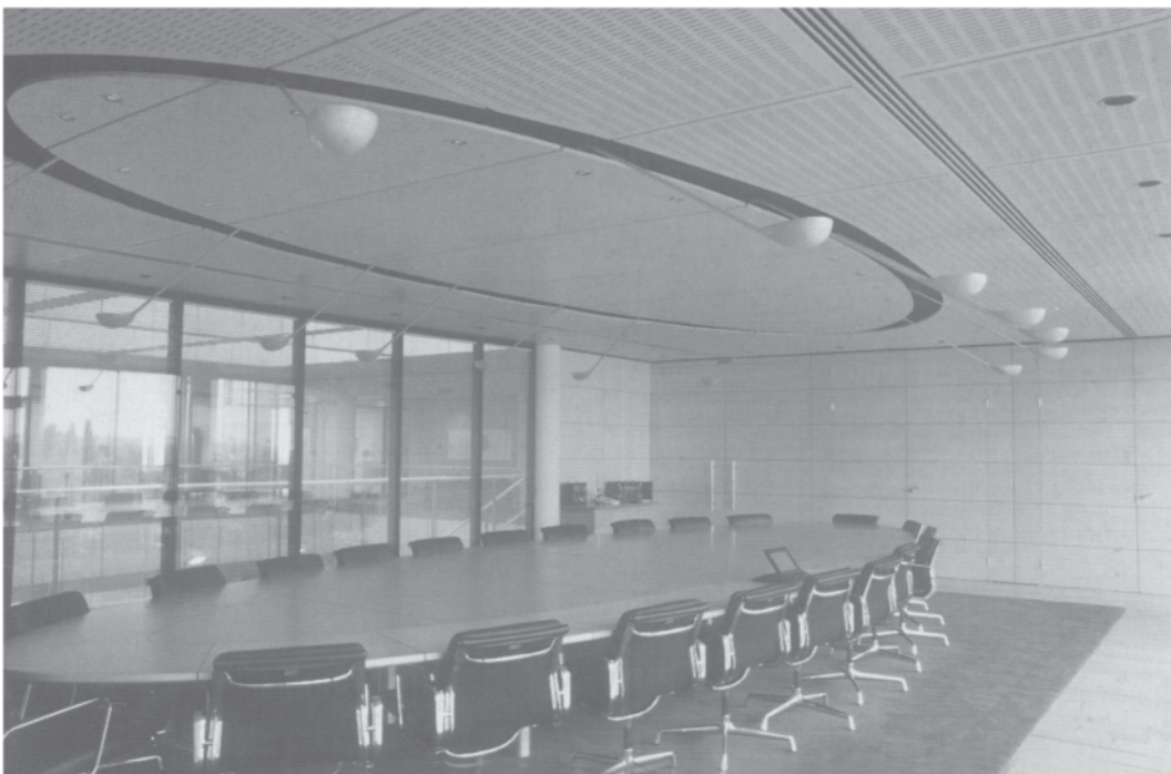
16.5 Board Room from the window side. Note the linear air supply diffuser in the ceiling and the glazed partition enabling a full view of the proceeding from the rest of the second floor.
