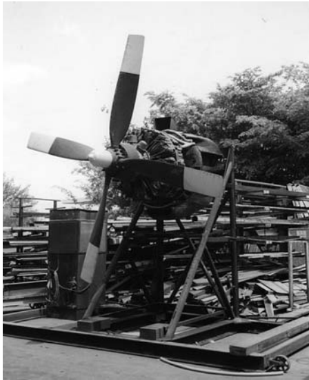
An airplane engine is used with a sprat rack for dynamic water infiltration mock-up testing.
