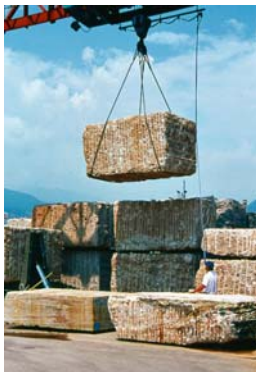
The granite blocks from the quarry were tested during the fabrication process. If results were below minimum specifications, the blocks were rejected.
