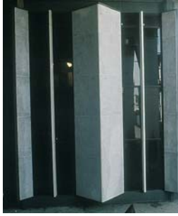
Mock-up of original Amoco Building façade at Construction Research Laboratory in Miami, Florida.
