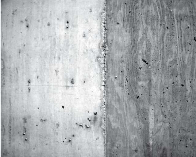
Fig. 5.2.2—Absorption of medium-density plywood (MDO) on left compared to regular plywood on right.
