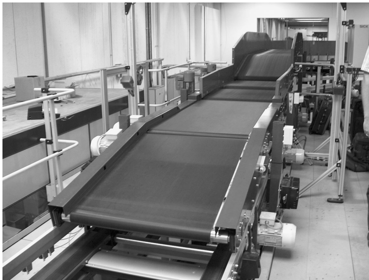
Figure 3.12 A toploader, where bags arrive on a traditional conveyor belt
