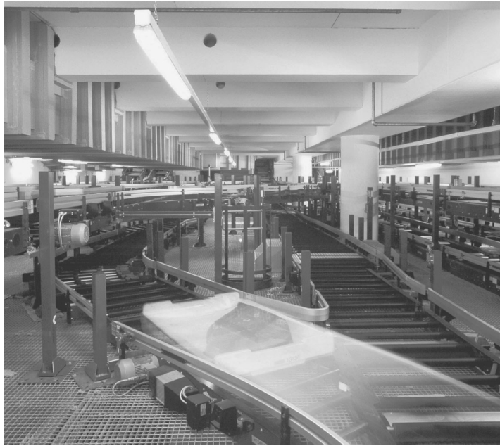
Figure 3.10 Snapshot into a BHS with a moving tote in the foreground
