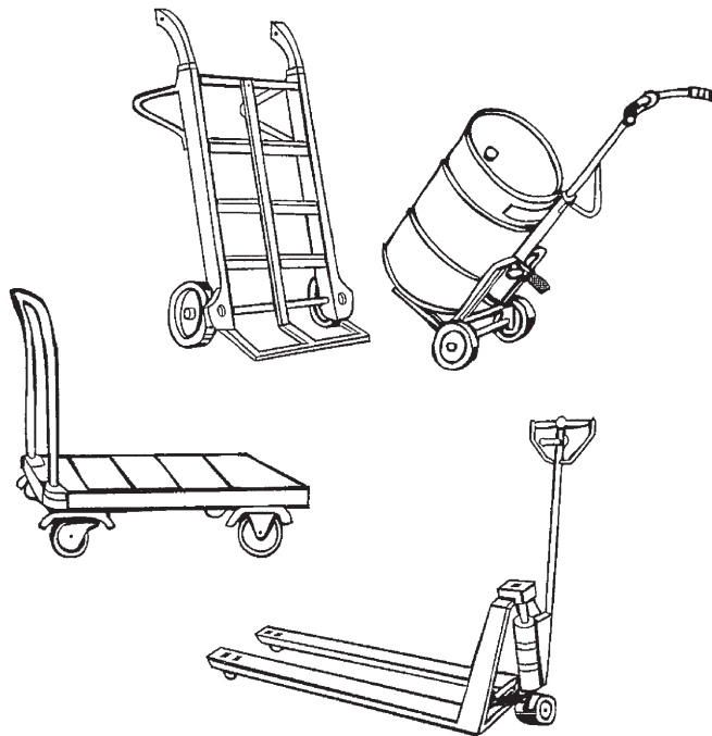
Figure 2.8 Typical hand trucks and carts used to transport materials (from Kroemer et al. 2001)
