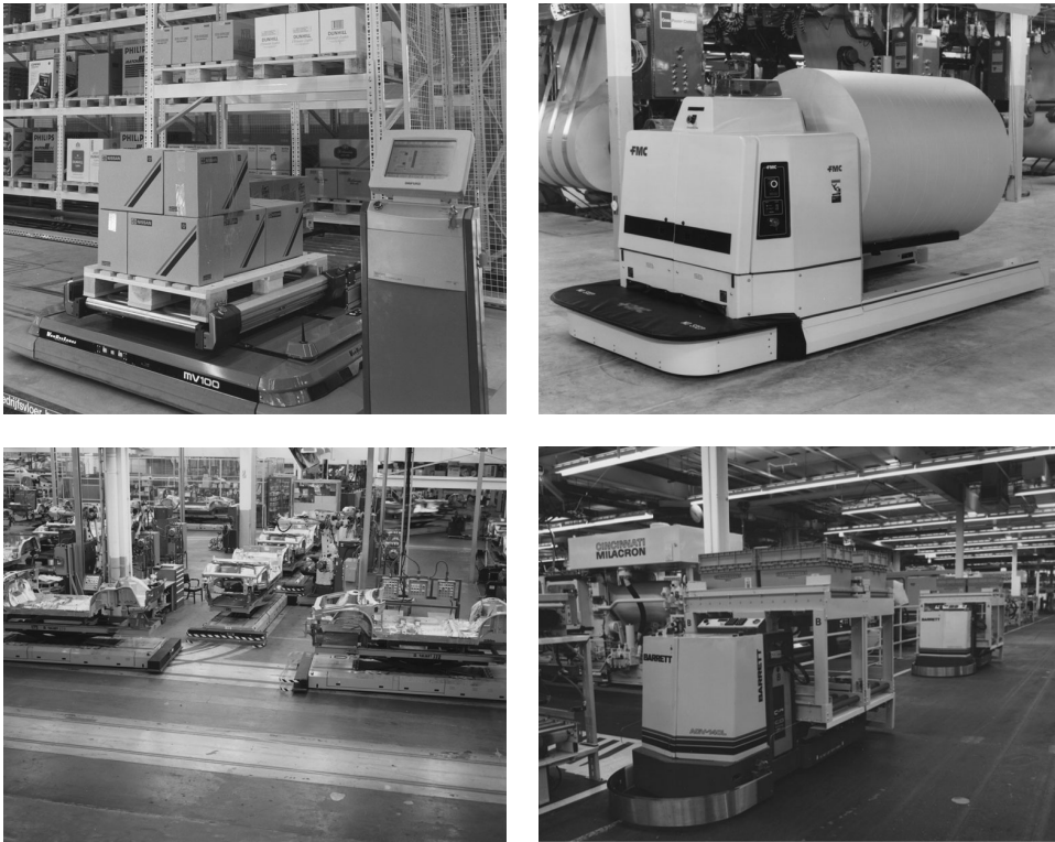
Figure 1.9 Use of AGVs in distribution and manufacturing activities (Source: Courtesy of Gould Communications)
