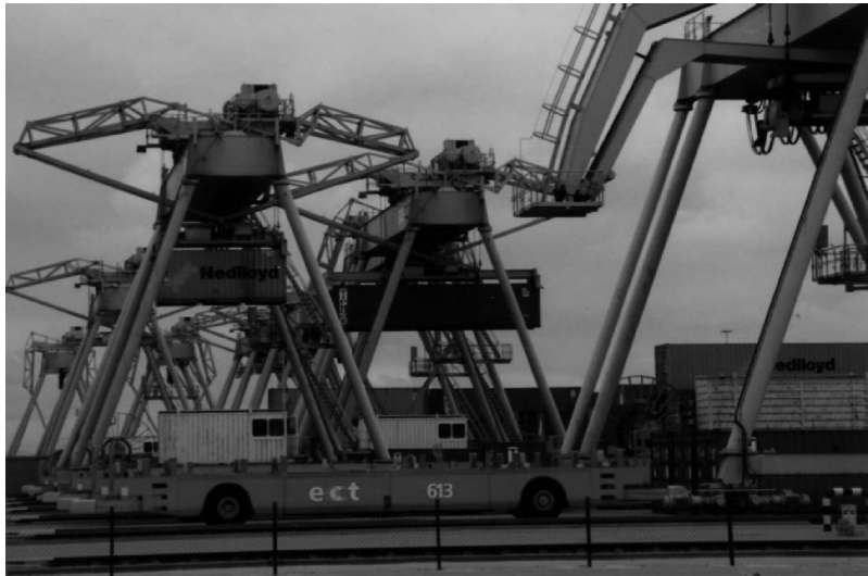
Figure 1.12 AGV and gantry crane used for loading containers on ships (Source: Courtesy of Europe Combined Terminals B.V., The Netherlands)
