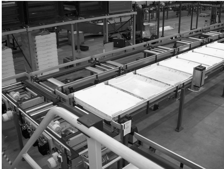
Figure 3.18 EBS elements, here storing a line of empty totes
