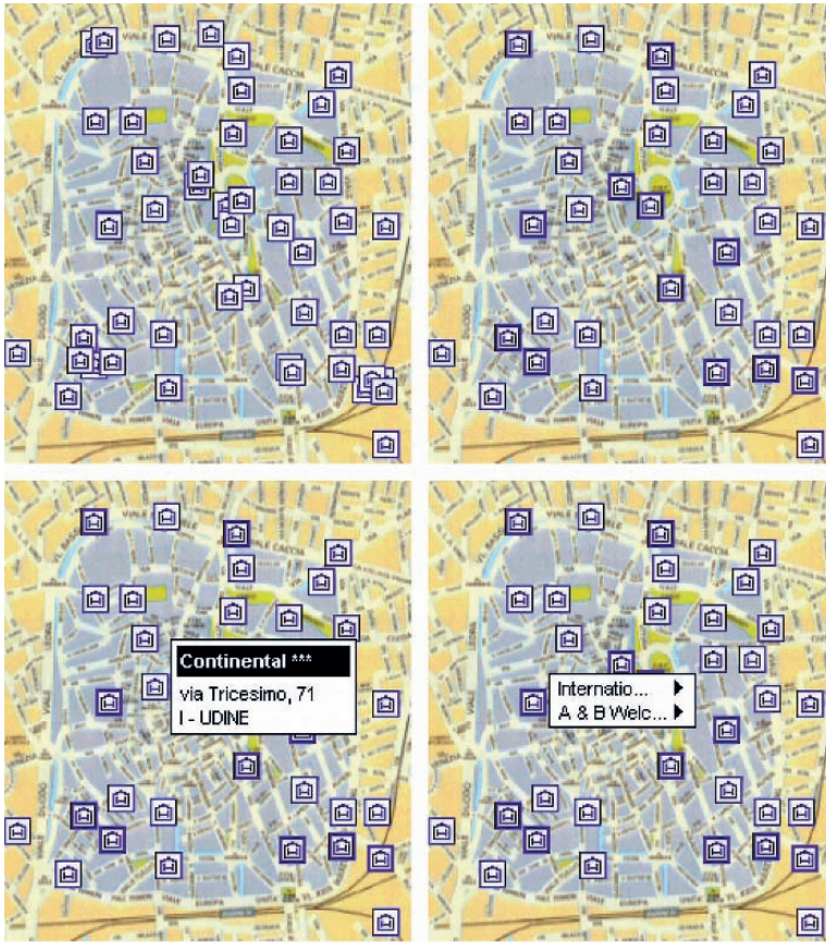
Fig. 2.4. An example of icon aggregation: all clusters of overlapping icons that can be seen in the original map visualization in the upper left image are replaced by special icons representing aggregations (as displayed in the upper right image). Selecting an individual icon allows one to obtain detailed information on the corresponding POI, while selecting an aggregator icon produces the list of aggregated POIs.
