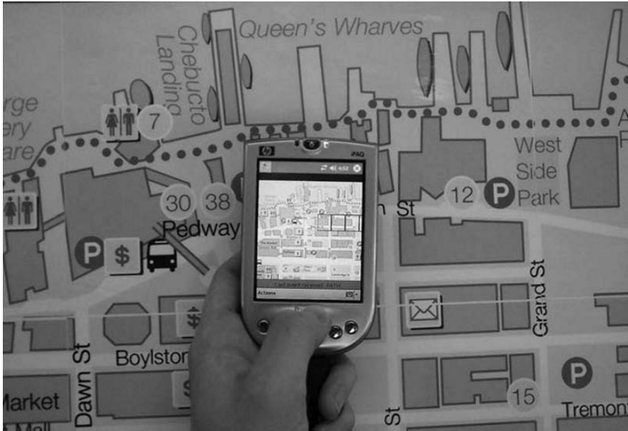
Fig. 13.2. A Marked-up map with PDA interaction. In this prototype RFID tags are placed in a regular grid on the other side of the paper map, and a reader on the PDA permits the user to select and interact with map regions.
