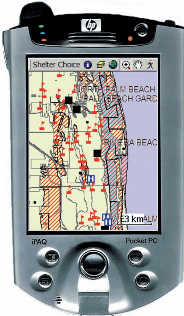
Fig. 16.5. User interface design for a mobile decision support system for emergency response – map of possible shelters (schools, hospitals). Source of map data: Florida Geographic Data Library, http://www.fgdl.org/ .
