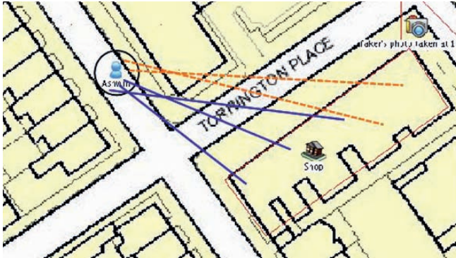
Fig. 14.4. Visibility computation for the filter -A random point is taken in the region around the reported position (the circle). Another random point is taken on the region (a building outline in this case), and ray is defined between them. The thicker rays hit the target while the thinner rays are obstructed by buildings in their path.
