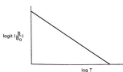
FIG. 8. Schematic logit–log plot used to linearize radioimmunoassay data. B and T are bound tracer and total antigen concentration, respectively, and B_0 is the value of B when no unlabeled antigen is added to tracer. The logit function is defined by Equation 40 , \text{logit}(Y) = \ln [Y/(1 - Y)] .
