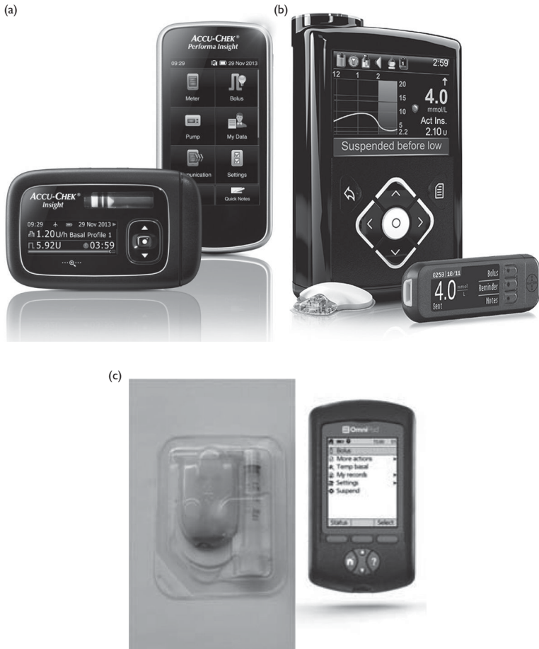
Figure 5.1 Some examples of insulin pumps. (a) Pump with remote control device: AccuCheck Insight (Roche); (b) Sensor-augmented pump: MiniMed 640G ® (c) ‘Patch’ pump: Omnipod (Ypsomed). Left, pump, replaced every 3 days. Right, handset.
