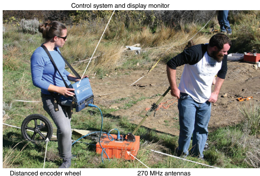
Figure 1.1 Collecting GPR profiles with a GSSI SIR-3000 control system and 270 MHz antennas.
