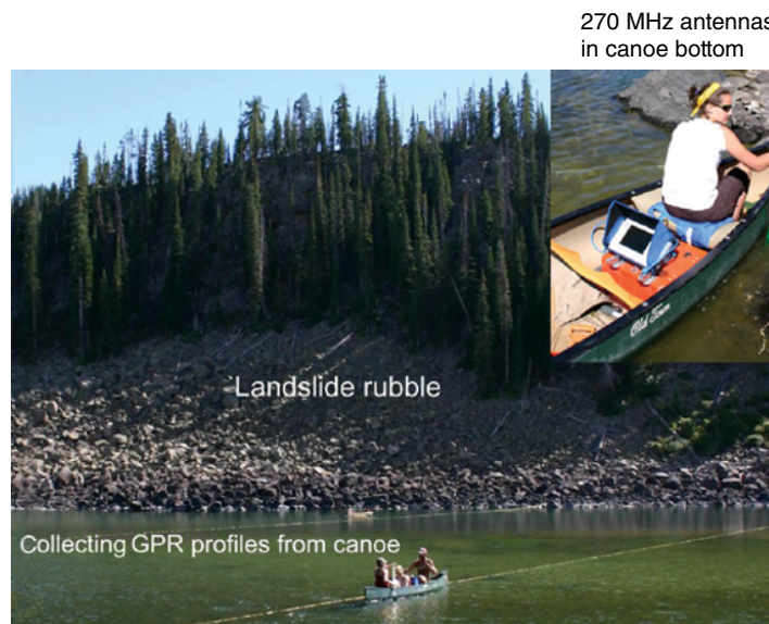
Figure 7.1 The 270 MHz antennae placed in the bottom of a canoe were used to collect reflection profiles as the boat was moved along a rope floating on the lake surface to assure linear transects. This lake at high elevation in the Rocky Mountains of
