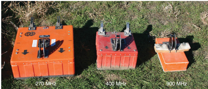
Figure 2.2 Some GPR antennae commonly used in ge archaeological investigations with the 270 MHz energy traveling deepest in the ground (up to 6 m), with the least feature and
