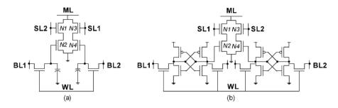
Figure 5-11. 6T dynamic TCAM cell (a), conventional 16T static TCAM cell (b).
