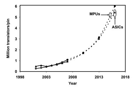
Figure 1-3. Number of transistors per IO pin for microprocessors and ASICs [22].
