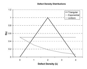
Figure 7-2. Defect Density Distributions.
