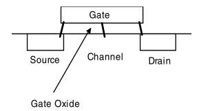
Figure 4-6. Structure of a MOS transistor and possible gate oxide short locations.
