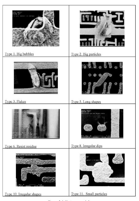
Figure 2-1. Various spot defects.
