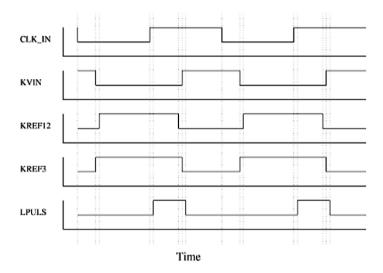
Figure 6-34. Input clock signal and various generated clocks in the analyzed flash A/D converter.
