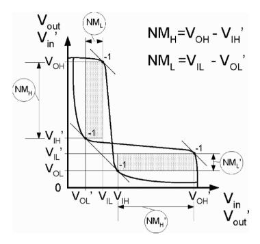
Figure 5-25. Graphical representation of SNM.
