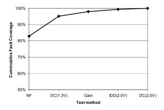
Figure 6-22. Optimized set of functional and structural tests.
