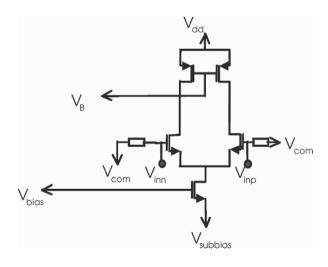
Figure 6-13. Low Noise Amplifier (LNA).
