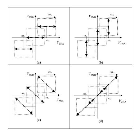
Figure 2-12.  $V_t$  mismatch analysis. (a) constant  $V_{tNB}$ , (b) constant  $V_{tNA}$ , (c)  $V_{tNA}$  and  $V_{tNB}$  running in opposite directions, (d)  $V_{tNA}$  and  $V_{tNB}$  running in the same direction.
