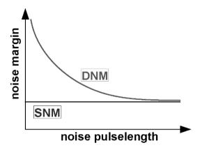
Figure 5-23. Noise margin with respect to noise duration.
