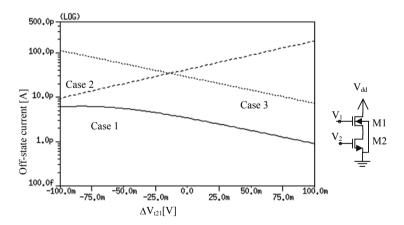
Figure 2-5. Leakage current as a function of  $V_t$  mismatch.
