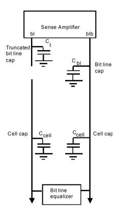
Figure 5-8. The stuck open fault.
