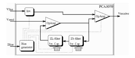
Figure 6-40. The antiside tone module of the PCA 1070.
