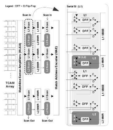
Figure 5-12. Scan chains for MMR testing.
