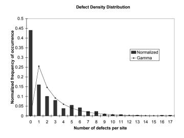
Figure 7-4. Fitting of Gamma distribution.
