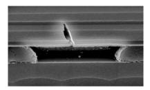
Figure 2-15. Open metal lines (a) Global top view of an open defect line. (b) Detailed cross-sectional view of the metal cavity and formation of the weak open defect due to the Ti barrier.
