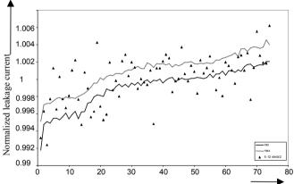
Figure 2-7. Impact of intra-die variations on leakage current. (a) expected correct behavior (b) intra-die variations of DSPs with leakage out of the tolerance window.
