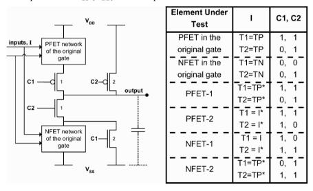
Figure 3-8. Robust SOP fault detection scheme and the 2-pattern test procedure [73].
