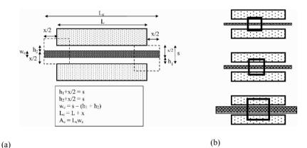
Figure 2-20. Critical area computation. (a) Setup and (b) Efect of defect size on critical area.
