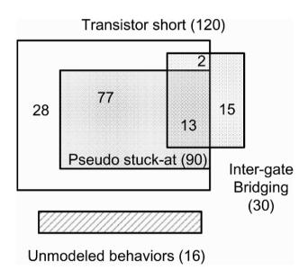
Figure 4-11. Overlap of faulty behaviours observed by Aitken [1].
