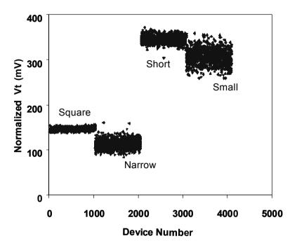
Figure 5-22. Normalized  $V_t$  for different sized transistors [courtesy Intel Corporation].
