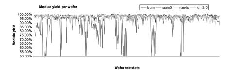
Figure 7-6. Module yield as a function of time.
