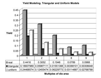
Figure 7-3. Yield modeling for triangular and uniform defect density models.
