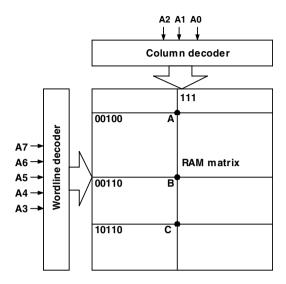
Figure 5-16. Graphical representation of the failure.
