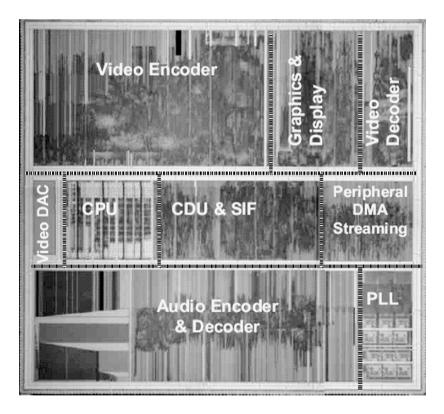
Figure 1-5. A typical systm on chip [17].
