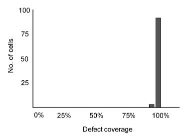
Figure 4-9. I<sub>DDO</sub> bridging defect coverage of a standard cell library [31].
