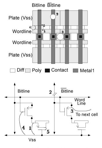
Figure 5-6. Physical defects in layout and their impact in schematic.
