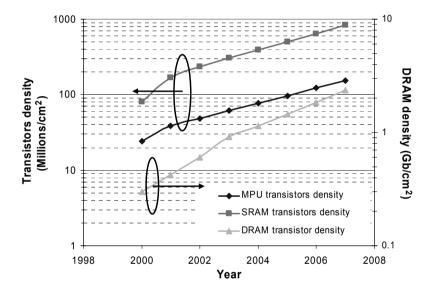
Figure 1-4. Growing transistor density [22].
