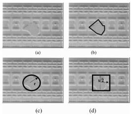
Figure 2-18. Modeling of spot defects.
