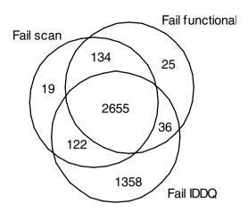
Figure 4-10. Distribution of failing die in each test class reported by Maxwell et al. [24].
