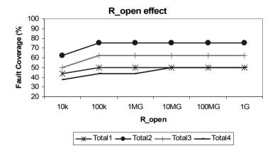
Figure 6-27. Fault coverage for weak opens.
