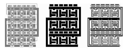
Figure 2-24. Layout sensitivity for open and short defect of each metal layer.
