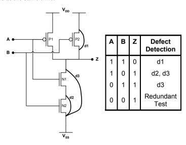
Figure 3-3. Defects in a 2-input NAND gate and their detection.
