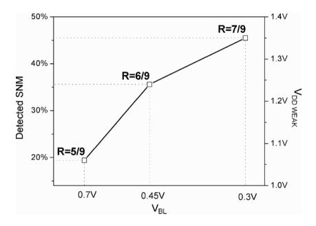
Figure 5-37. Measured detection capability of the programmable RCRT.
