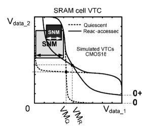
Figure 5-28. Simulated SRAM cell transfer characteristics under quiescent and read access conditions.
