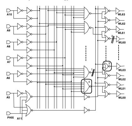
Figure 5-19. A typical wordline address decoder.
