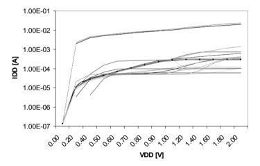
Figure 6-18. Current signatures for the first 50 bridges.
