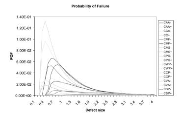
Figure 2-26. Probability of failure for each defect type.
