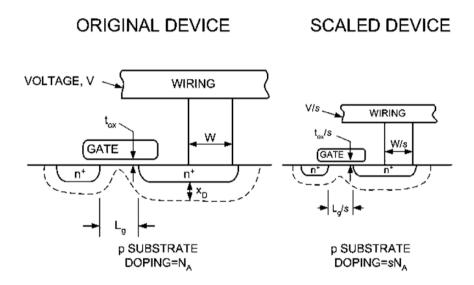
Figure 1-1. MOS transistor scaling.
