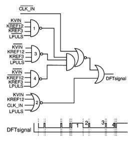
Figure 6-35. A DfT scheme for testing clock generator faults in the analyzed flash A/D.
