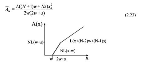
Figure 2-30. Critical area of N conductors.
