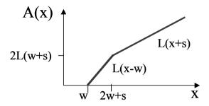
Figure 2-28. Critical area for two conductors.
