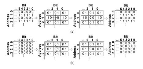
Figure 5-13. Data patterns to stimulate (a) horizontal/vertical and (b) diagonal inter-cell faults.
