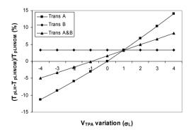
Figure 2-9. Delay for  $V_{tPB}$  constant and greater than the nominal value ( $V_{tPBNOM}$ ).
