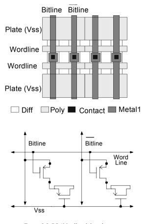
Figure 5-5. DRAM cell and the schematic.
