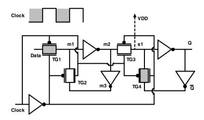
Figure 4-13. A bridging defect between s1 and  $V_{DD}$  in a typical CMOS flip-flop is not detected by  $I_{DDO}$ .
