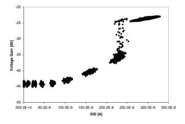
Figure 6-17. Correlation of  $I_{DDO}$  against voltage gain for various power supply voltages.
