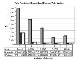
Figure 7-1. Yield prediction for binomial and Poisson models.
