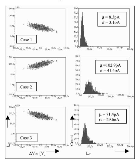
Figure 2-6. Monte Carlo simulations to estimate intra-die off-state current. Scatter plots present points for off-state current vs.  $V_t$  mismatch. Histograms show the corresponding distribution of off-state currents.
