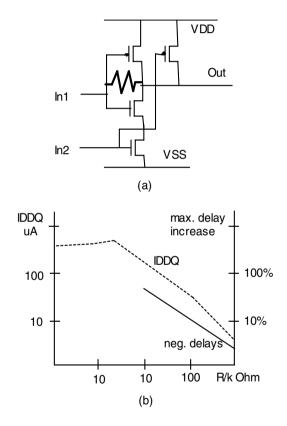
Figure 4-12. A bridging fault improving logic delay of a two input NAND gate [47].
