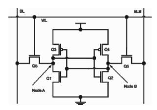
Figure 5-24. The 6T SRAM cell.
