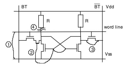
Figure 5-2. Examples of defects for different fault classes.
