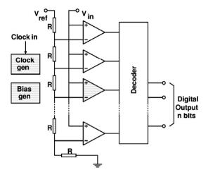
Figure 6-32. Block diagram of a flash A/D converter.
