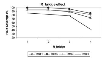
Figure 6-25. Fault coverage for "weak" bridges.
