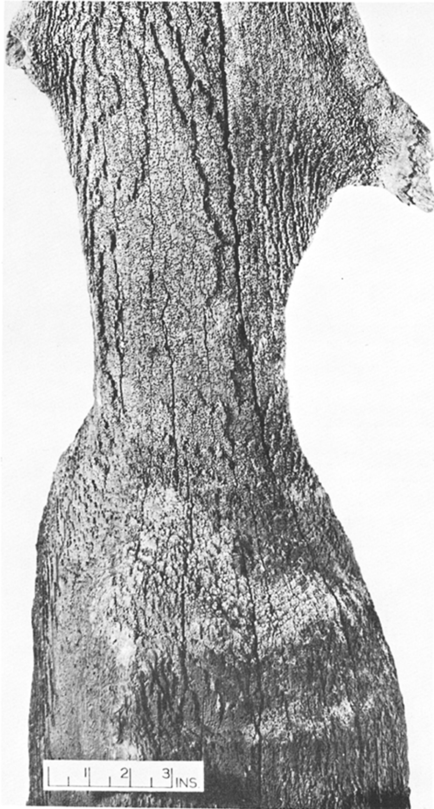
Fig. 10.2 (b) Attack by limnoria (Crown copyright reproduced with permission of BRE, Princes Risborough Laboratory)
