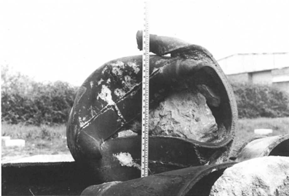
Fig. 2.24b Buckling and tearing of welded-on external stiffening ring to tubular steel pile driven on to sloping rock surface
