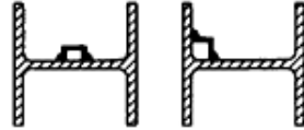
Fig. 2.20 Ducts welded to webs of H-section piles for measurements of curvature by inclinometer
