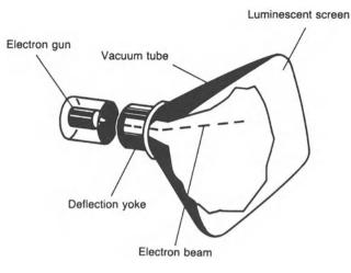
FIGURE 15.1. Cathode ray tube.
