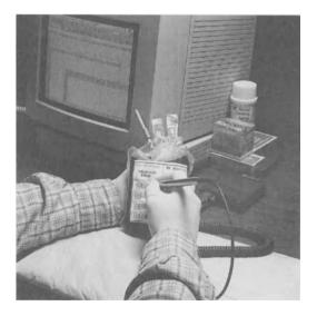
FIGURE 7.5. Bar code reader. (Photograph courtesy of Prologix.)
