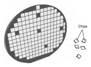
FIGURE 2.1. Silicon wafer.
