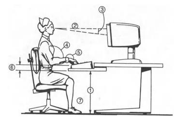
**FIGURE 15.2.** NIOSH specifications for VDT use show: (1) height of keys at 29–31 inches, (2) optimal viewing distance 17–25 inches, (3) screen center 10–20 degrees below plane of operator's eye height, (4) angle between upper and lower arm 80–120 degrees, (5) wrist angle under 10 degrees, (6) keyboard at or below elbow height, (7) ample leg room. (From *Computers and Medicine* 2, no. 5 (September 1982).)
