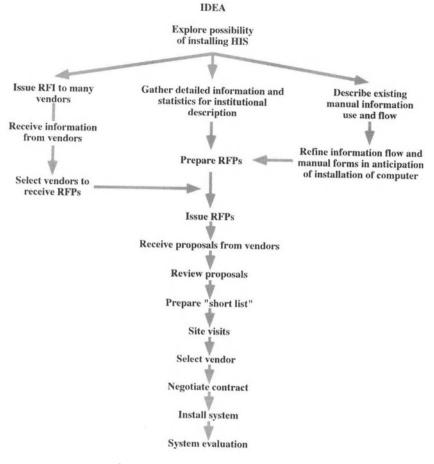
FIGURE 13.1. Hardware and software selection process.
