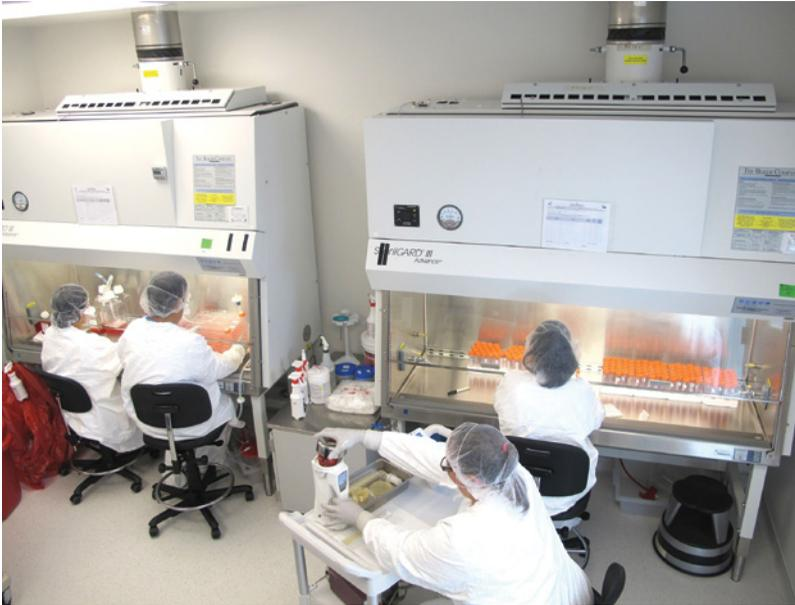
**Figure 7.6** Vector manufacturing. Showing the interior of a Class 10,000 (ISO 7) manufacturing suite during retroviral vector production. Staff at the left-hand BSC are harvesting the supernatant. The staff member
