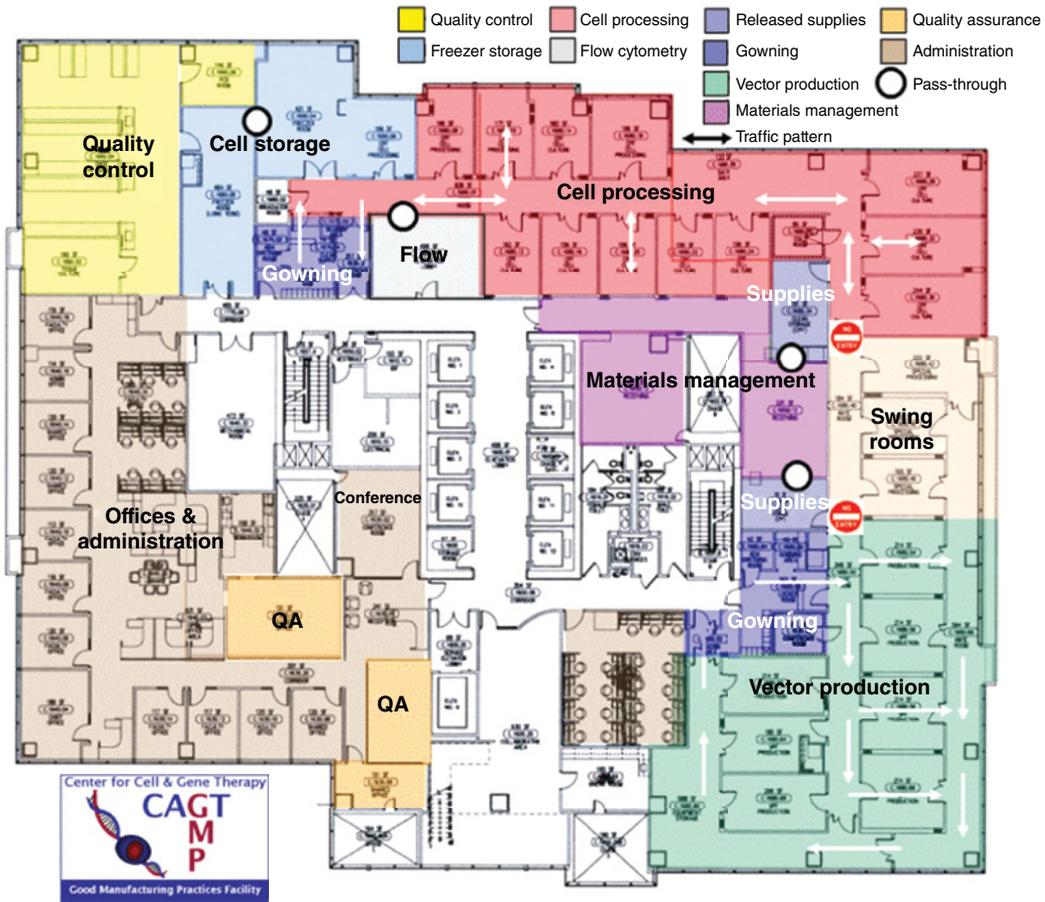
**Figure 7.5** Floor plan of the cGMP facilities at the Baylor Center for Cell and Gene Therapy. The Vector Production Facility has unidirectional flow of staff, materials,
