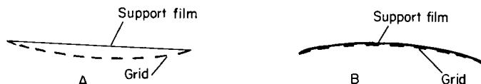
FIG. 3. (A) Grids presenting a concave surface may result in the film making contact only at the periphery of the support. Stability of the support films can be improved by ensuring that the maximum contact with the grid bars takes place as shown in (B).
