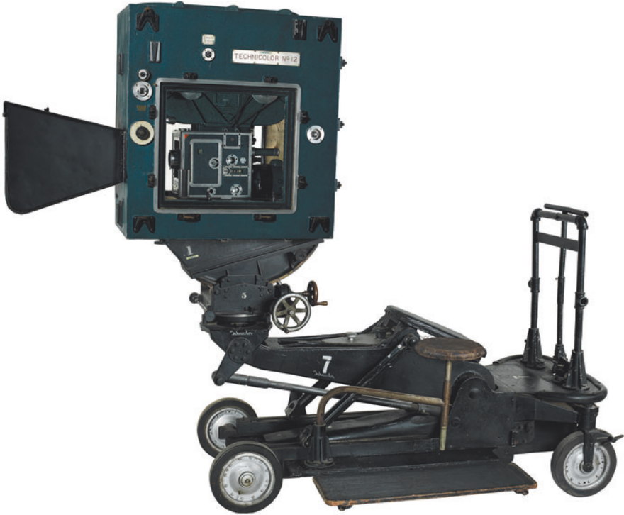
Fig. 7.3 Technicolor camera encased in a sound-dampening blimp, used in the filming of The Wizard of Oz
