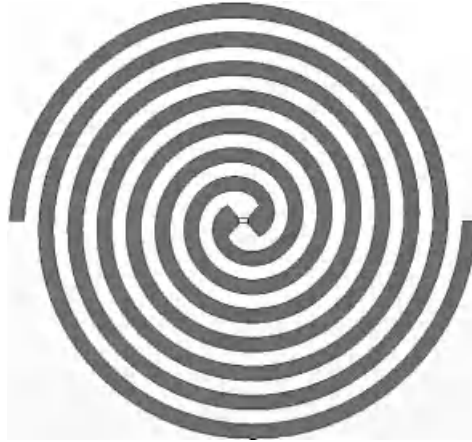
Figure 17.4 Archimedean spiral antenna.
