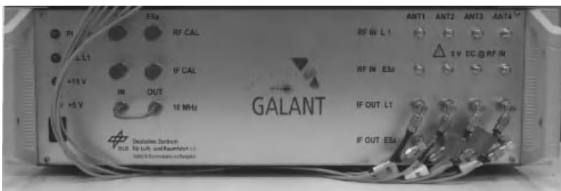
Figure 9.21 E1/E5a RF front-end.
