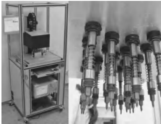
Figure 2.32 A photo of the IAFTT robot controlling all tuning elements simultaneously.
