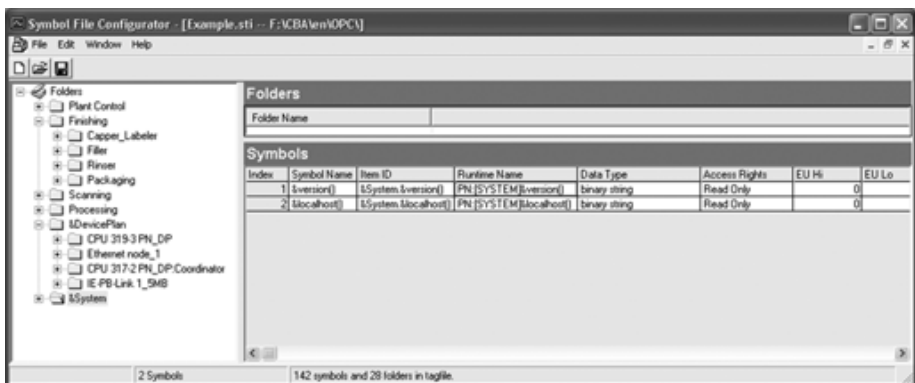
Fig. 5.65 System variables in the Simatic Net symbol file configurator
