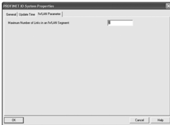
Fig. 4.32 Setting of IWLAN parameters with Profinet IO Systems
