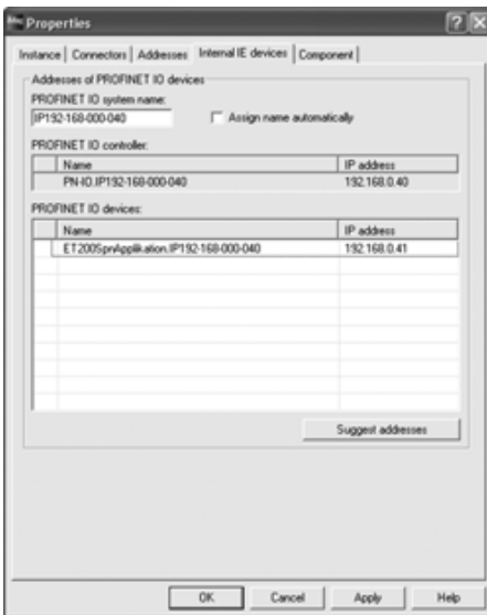
Fig. 5.50 Properties of internal IE devices
