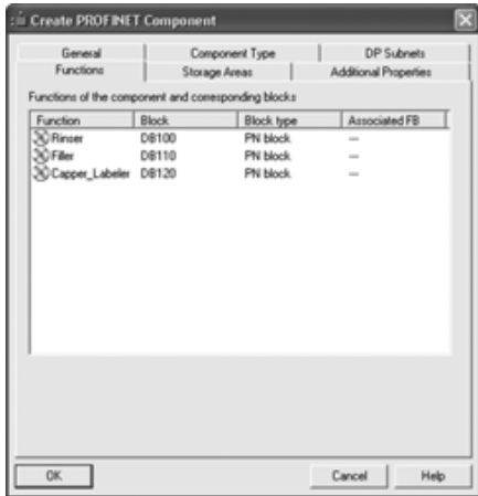
Fig. 5.40 Display of the functions of a Profinet component
