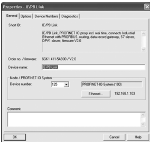
Fig. 4.36 General settings of the Simatic Net IE/PB Link PN IO and IWLAN/PB Link PN IO gateways
