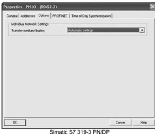
Fig. 4.25 Setting of options for PN IO interfaces with Simatic S7
