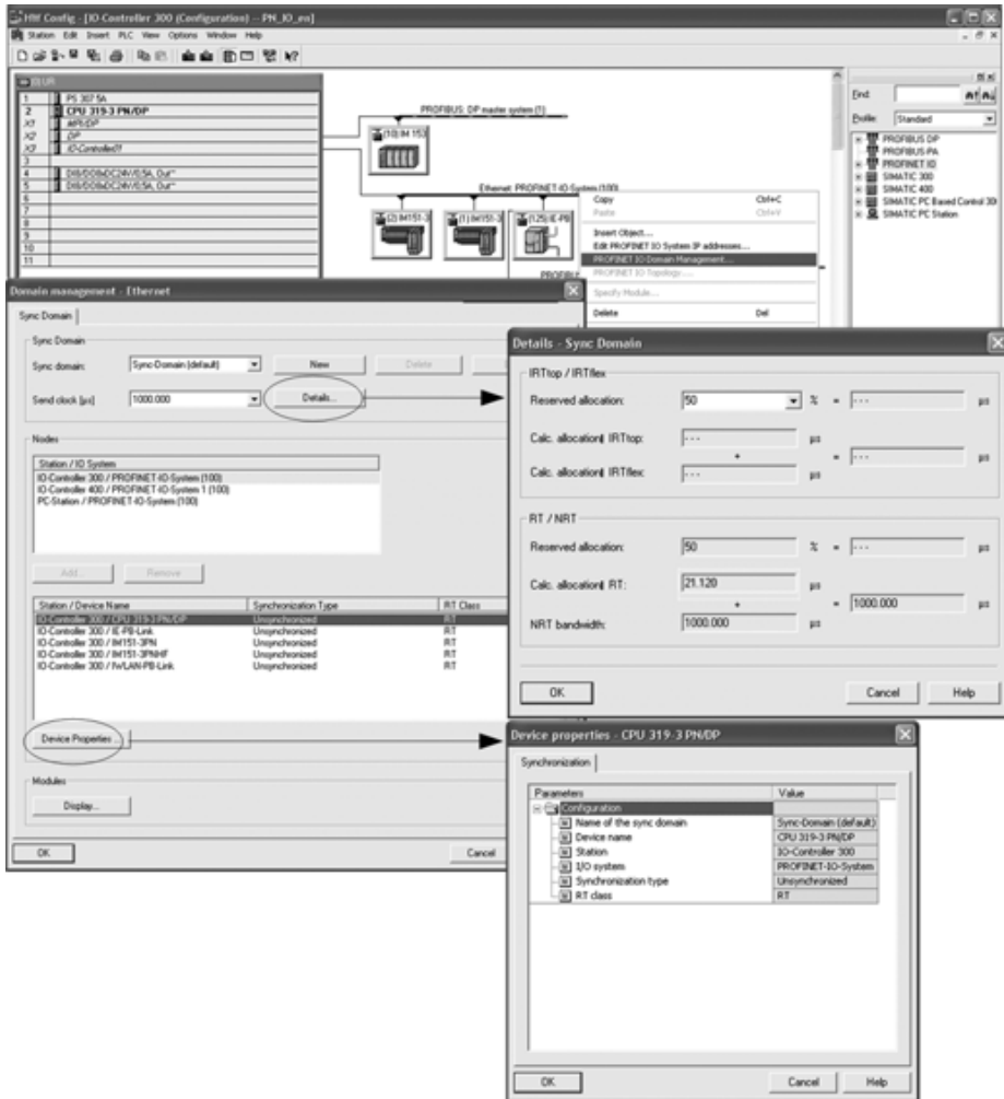
Fig. 4.41 Parameters in the window “Device properties”, tab “Synchronization”
