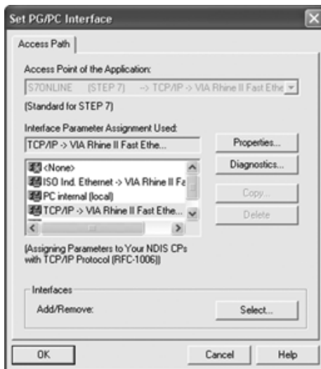
Fig. 5.57 Setting of PG/PC interfaces
