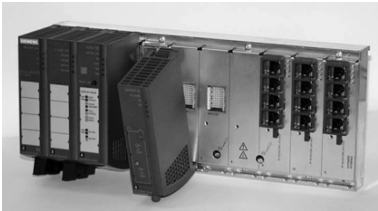
Fig. 7.50 Basic device without media modules, caps and covers
