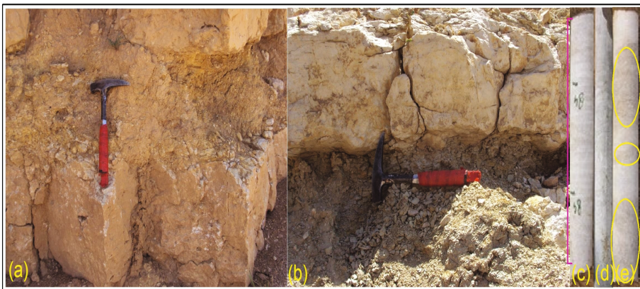
Fig. 2. Lithological variations in the samples: (a) limestone (b) argillaceous limestone (c) Alternate bedding of limestone and argillaceous limestone (d) Alternate bedding (e) Encircled part is argillaceous limestone
