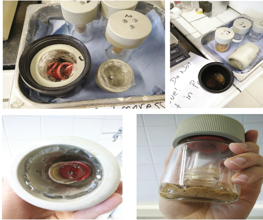
Fig. 9. Pictures showing broken chambers and sample tubes at higher speeds (>2400 RPM)
