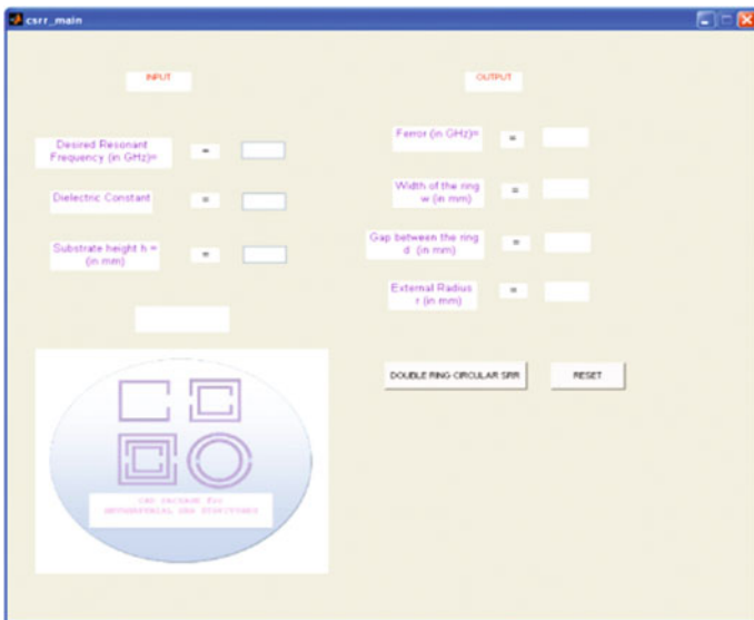
Fig. 2.10 Graphical user interface of PSO-based CAD package for design of metamaterial structures
