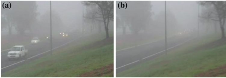
Fig. 29.2 Background extraction example: a the first original haze frame from video. b Background image obtained by frame differential method
