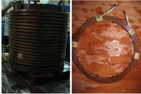
Fig. 39.5 The laboratory winding and the deformed discs
