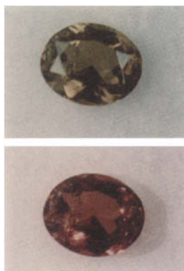
Color plate 11. A synthetic alexandrite gemstone, 5 mm across, changing from a reddish color in the light from an incandescent lamp to a greenish color in the light from a fluorescent tube lamp. Photograph K. Nassau.
