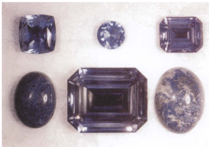
Color plate 12. Six blue gemstones with different causes of color. Left to right: above: Maxixe-type beryl (radiation-induced color center), blue spinel (ligand field color from a Co impurity), spinel doublet (colorless spinel containing a layer of organic dye); below: shattuckite (ligand field in an idiochromatic Co compound), blue sapphire (Fe-Ti intervalence charge transfer); lapis lazuli ( \text{S}_3^- anion-anion charge transfer); the largest stone is 2 cm across. Photograph K. Nassau.
