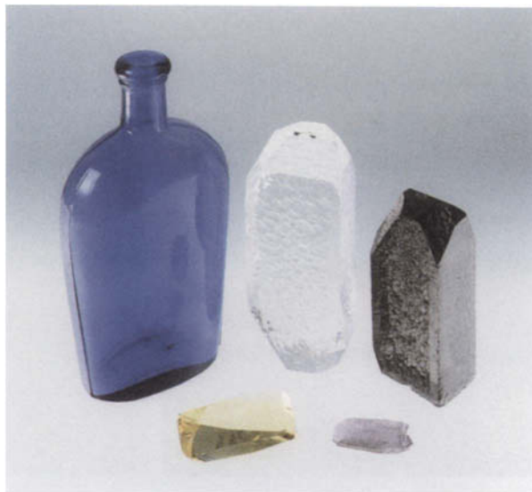
Color plate 17. Irradiation-produced color centers. Left to right: above: century-old glass bottle irradiated to form desert amethyst glass, a colorless synthetic quartz crystal as grown, and one that has been irradiated to form smoky quartz; below: a man-made citrine quartz colored yellow by Fe, and one that has been additionally irradiated to form the amethyst color center. Photograph K. Nassau.
