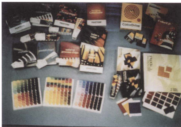
Color plate 7. Examples of collections of colors consisting of ink on paper, paint on paper, dyed textiles, and plastic chips that are used for the specification of color. Courtesy of Pantone, Inc.
