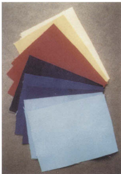
Color plate 32. Ten samples of polyester fabric colored with the disperse dyes of fig. 6.11(b). Samples courtesy of Ciba Speciality Chemical, Textile Products Division, Photograph by Kurt Nassau.
