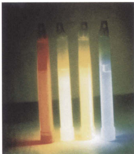
Color plate 13. Four chemoluminescent “Cyalume” light sticks, 15 cm long, made by the American Cyanamid Company. Photograph K. Nassau.
