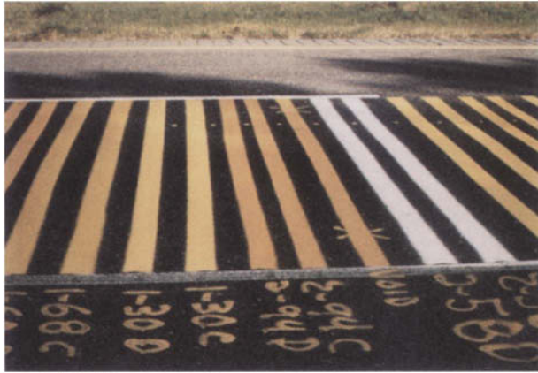
Color plate 29. Road testing of traffic-marking paints using the monoarilide pigment Yellow 65. Note that the stripes are oriented across the road so as to receive maximum wear. Courtesy of Sun Chemical Corp.
