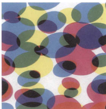
Color plate 33. The white, yellow, magenta, cyan, red, green, and blue (black has been omitted for clarity) micro areas that are fused or blended by the eye when evaluating a photomechanical reproduction. (This should also be judged from far enough away so that fusion occurs.) Courtesy Graphic Arts Technical Foundation.
