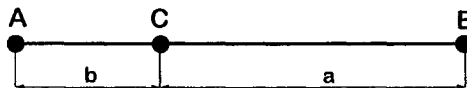
Fig. 1.8. The law of the lever; mixing amount a of color A with amount b of color B results in color C on the chromaticity diagram of fig. 1.7.
