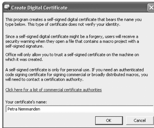
FIGURE 18-4 Use the Digital Certificate for VBA Projects applet to create your own digital certificate for testing purposes.
