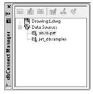
You can dock and undock the dbConnect Manager like any palette. You can also resize it by dragging its right border left or right. After you open the dbConnect Manager, you see a list of open drawings and configured data sources.
