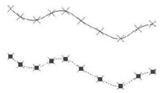
Because the spline is calculated based on the control points, the fit points are not necessary to generate the spline. In fact, if you use the Move vertex or Refine options to move or edit a control point, only the control points are needed to generate the spline, and the fit point information is discarded so that you can no longer edit it. The Fit Data option also disappears from the prompt. You can edit the fit points by using grips.
