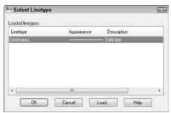
If the linetype that you want appears on the list, click the linetype and choose OK to close the dialog box. If the linetype does not appear, you need to load the linetype. Click Load to open the Load or Reload Linetypes dialog box, as shown in Figure 11.6.
