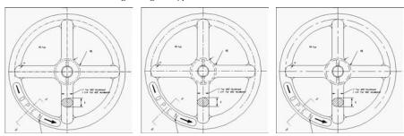
For purposes of drawing, you simply want to make sure that you can distinguish the linetype both when you can see the entire drawing on the screen and when you zoom in close. The main reason to scale linetypes is for plotting. A linetype scale that works for a drawing of a house on-screen may appear continuous when you plot it at a scale factor of 1 = 96.
