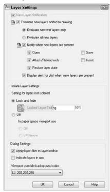
By default, layer notification only applies when xrefs add new layers to a drawing, because xrefs are the most common means of adding layers without your knowledge. However, you can choose the Evaluate All New Layers option, especially if you use templates that already contain all the desired layers.
