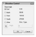
Here you can choose to have 0 degrees start in a direction other than East. You can also choose Other and type any other angle or click the Pick an Angle button to pick two points on your screen that specify an angle. Click OK to close the Direction Control dialog box. Click OK to close the Drawing Units dialog box.
