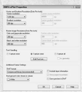
When you finish specifying the properties for the DWF file format, click OK. If you see a message asking whether you to apply the changes for the current plot only (which creates an override of the configuration file but doesn't change it) or to save the changes to the file (which changes the configuration file, although you can always change it back), respond as desired.
