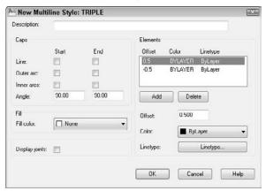
The Elements section lists the current elements of the multiline. Elements are the lines that make up the multiline. The offset defines the distance of the line from the start point when you start to draw. An offset of zero places the line on the start point. As you can see, the Standard multiline style has two elements, each 0.5 units from the start point. Figure 16.26 shows the Standard multiline style as it appears in relation to the start point that you pick.
