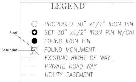
The base point does not have to be on the object, but it should be in a location that makes it easy to insert the block. Figure 18.2 shows a different sort of block, a title border/block. In this case, the base point is usually inserted at 0,0 of the drawing. By placing the base point at the lower-left corner of the border, you can easily place this block in any drawing. The base point is similar in concept to the justification point on text objects.
