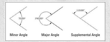
Here's how you create each type of dimension. Start the DIMANGULAR command. The command responds with the Select arc, circle, line, or <specify vertex>: prompt.
