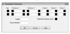
Use this dialog box to build the frame. The frame enables you to create two rows of two tolerances and three datum references (for up to three dimensions), as well as a projected tolerance zone value and a symbol and datum identifier. You'll rarely, if ever, use all the features in the frame.
