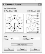
When you open the dialog box, the black needles indicate the angles for the current view. When you change the angles, the black (or white) needles move to the new angle, but the original needle remains to indicate the current angle. This enables you to constantly see the current angles for reference.
