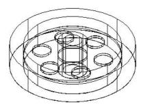
Figure 22.31 shows the result of SOLPROF after also freezing the layer that SOLPROF created which contains the hidden parts of the model. In this case, the layer was named PH-159. Look for the *H*, which stands for hidden. The last part of the layer name is the handle of the object that you're profiling, so it differs for each object.
