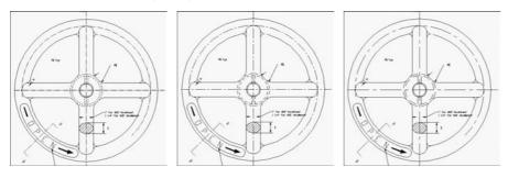
For purposes of drawing, you simply want to make sure that you can distinguish the linetype both when you can see the entire drawing on the screen and when you zoom in close. The main reason to scale line-types is for plotting. A linetype scale that works for a drawing of a house on-screen may appear continuous when you plot it at a scale factor of 1=96.
