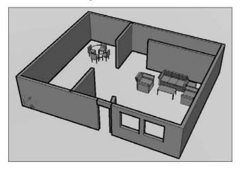
You can use the Close option to close the polysolid. You can also use the Justify option to determine whether the polysolid is centered around the points you specify (the default), left-justified (your points are to the left side if you're drawing upward), or right-justified.
