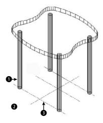
12. Choose Home tab ⇒ Properties panel ⇒ List. Select the front-left leg at 1, shown in Figure 21.20. Press Enter. The center (of the circle at the bottom of the leg) is X = 3.5000, Y = -7.0000, Z = 0.0000.
