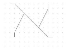
Planning in advance is almost essential. A common technique is to draw the shape in a drawing on a grid set to 1-unit spacing. You can use only integers in your shape codes, so you must often scale the shape up so that the smallest line segment is 1 unit.
