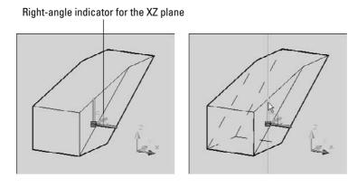
**2.** Pass the cursor over any grip (but not an arrow); the move grip tool jumps to that grip, as shown on the left side of Figure 24.33. This temporarily places the origin of the UCS at that point.
