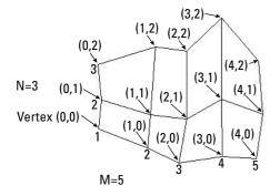
After you set the size of the 3D Mesh, you need to specify each vertex. For example, the 3D Mesh in Figure 23.12 has 15 vertices that you need to specify. AutoCAD prompts you for each vertex in order, starting with (0,0). Vertex (0,1) is the second vertex in the first column. Vertex (1,0) is the first vertex in the second column, starting from the bottom. It's a little confusing because AutoCAD starts the counting from 0 (zero), not 1. For the 3D Mesh in Figure 23.12, the last vertex is (4,2).
