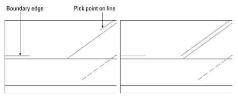
You can extend arcs, elliptical arcs, lines, open polylines, and rays. You can use polylines, arcs, circles, ellipses, elliptical arcs, lines, rays, regions, splines, text, or xlines as boundary edges. An object can be used as both a boundary edge and an object to be extended in the same extending process.
