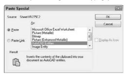
The choices that you see in the As box of the Paste Special dialog box depend on the type of data that you copied. In most cases, you can paste as an object of the source application, as a picture (metafile), as a bitmap, and as text. Table 27.3 describes the characteristics of the choices that are available in the example in Figure 27.11.
