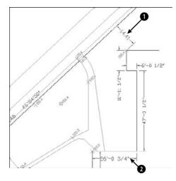
AUTOCAD ONIN The Express Tools command, DIMREASSOC, does the same thing that you accomplished in Step 3 of this exercise — restoring the default measurement value to modified dimension text. Choose Menu Browser 🗘 Express 🗘 Dimension 🖒 Reset Dim Text Value.
