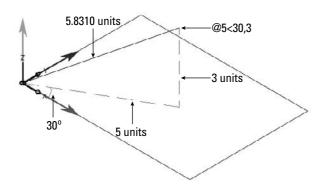
Spherical coordinates have the format (@)distance<angle<angle:
