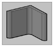
The mounting angle should have two holes in it. You would create the holes using the SUBTRACT command, which I cover later in this chapter.
