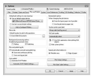
In the Default Plot Settings for New Drawings section, you set the default plotter/printer for new drawings and whether or not to use the same settings that you used the last time you plotted. As soon as you create plot settings for a drawing, those settings are saved with the drawing. Click Add or Configure Plotters for access to the Add-a-Plotter Wizard and existing plot configuration files. If you use a template, the plot settings in the template take precedence over the settings here.
