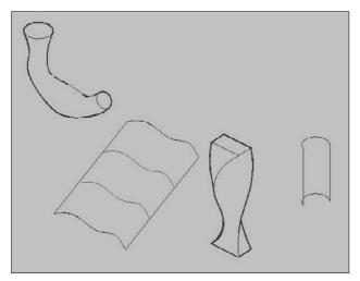
The difficult part of lofting is drawing and placing the source cross-sections to get the result that you want. To create a lofted surface or solid, follow these steps:
