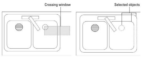
BOX: The BOX option is a combination of the Window and Crossing options. If you pick the two window corners from left to right, the selection functions as if you used the Window option. If you pick the two points from right to left, the selection functions as if you used the Crossing option. By default, you can select objects this way without specifying the BOX option. See the description of implied windowing later in this chapter.
