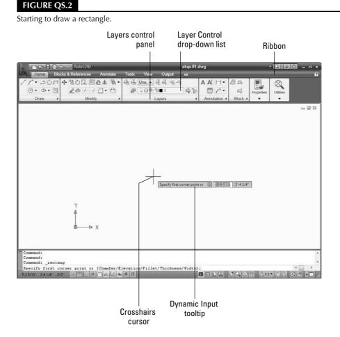
You see the full prompt shown here in the Command window at the bottom of your screen. You see an abbreviated version of the same prompt in the Dynamic Input tooltip that appears near the mouse cursor. In an architectural drawing, distances are assumed to be in inches, so you don't need to specify a unit (although you can if you want).
