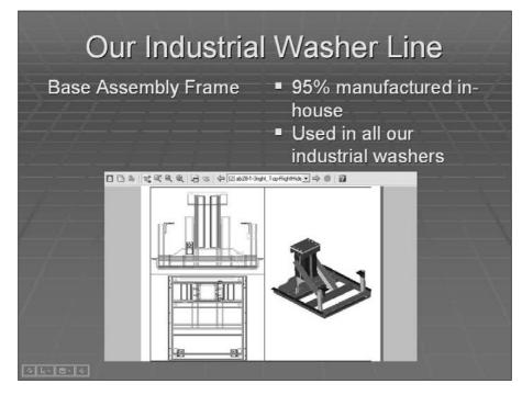
You can hide a 3D view and copy and paste the view into another application. However, you cannot copy and paste a rendered view. To bring a rendered view into another application, save it as an image and import it. Chapter 25 covers saving rendered images. You can freeze any layers that you don't want to include, such as dimension and text layers.
