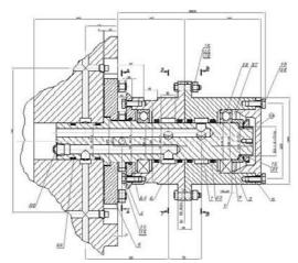
Thanks to Vladimir Sevastyanov of Ukraine for this drawing of a gyrating swivel that feeds oil to an uncoiling machine used in the cold rolling of metal.
