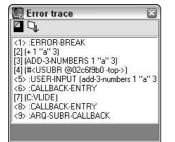
The item numbered <5> in Figure 36.1 is what you entered in the Console. The item labeled [2] (+ 1 "a" 3) is where the error occurred, while <1> : ERROR-BREAK signaled the function's termination because of the error.
