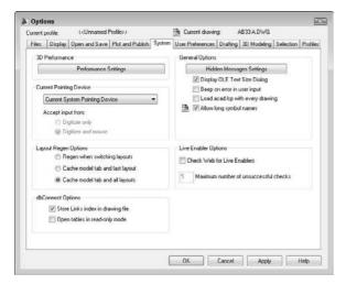
In the 3D Performance Settings section (AutoCAD only), click the Performance Settings button to open the Adaptive Degradation and Performance Tuning dialog box, shown in Figure A.7.
