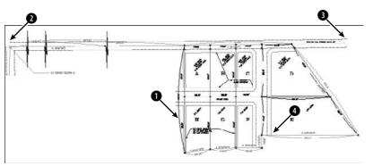
3. Choose Tools tab \$\dots\$ Inquiry panel \$\dots\$ Distance. At the Specify first point: prompt, choose the endpoint at 2, shown in Figure 12.5, using the Endpoint running object snap. At the Specify second point: prompt, choose the endpoint at 3. Here's the result:
