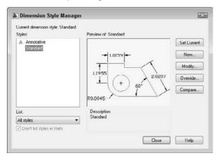
To create a new style, click New to open the Create New Dimension Style dialog box, shown in Figure 15.2. Type a new name in the New Style Name text box. In the Start With drop-down list, choose which existing dimension style you want to use as a basis for the new dimension style. If you have more than one to choose from, choose the style that most resembles the new style you want to create.
