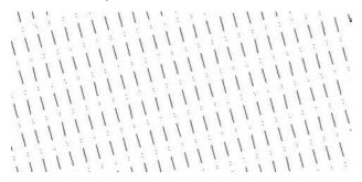
If you add a delta-x of 0.25, the lines in the pattern are staggered by 0.25 units, along the direction of the lines, as shown in this code and in Figure 31.8:
