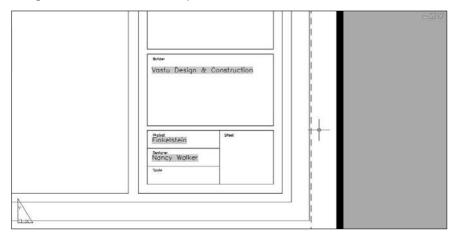
By default, a field is evaluated and updated, if necessary, whenever you open, save, plot, eTransmit, or regenerate a drawing. (See Chapter 28 for information on eTransmitting a drawing.) You can change when AutoCAD updates a field by choosing Menu Browser ➡ Tools ➡ Options, and clicking the User Preferences tab. In the Fields section, click Field Update Settings. Check or uncheck the items that you want, and then click Apply & Close. Click OK to close the Options dialog box.
