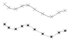
To edit a spline, choose Home tab r Modify panel (expanded) Jdit Spline to start the SPLINEDIT command. After you select the spline, the command responds with the Enter an option [Fit data/Close/Move vertex/Refine/rEverse/Undo]: prompt. Here's how to use these options:
