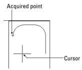
**3.** Move the cursor away from the object snap toward your desired point. You see the temporary alignment paths as you move the cursor over available drawing paths, as shown in Figure 4.24. If Ortho Mode is on, you see only horizontal and vertical paths. If Polar mode is on, you see polar paths based on the polar angle settings, as explained earlier in this chapter.
