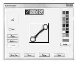
The center of the editing area shows an enlarged view of the button. You see the button's actual size at the top-left corner of the dialog box. Check the Grid check box to show a grid of pixels — this is just a drawing aid. Choose a color from the color palette and then choose one of the four tools at the top of the dialog box:
