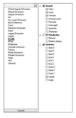
The general properties listed when no object is selected in the object list apply to all objects, even objects not on the object list. For example, a spline is not on the list by default. Therefore, if you select a spline, you'll see only Color and Layer properties, which are the default general properties for all objects. By adding an object to the list, you can specify which additional properties you want to see for that object type.
