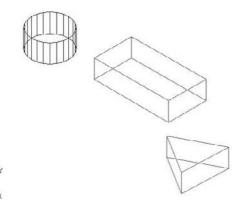
Surfaces created by adding thickness are sometimes called 2½D objects. Although they have three dimensions, the third dimension can only be a straight side perpendicular to the 2D object at the base.
