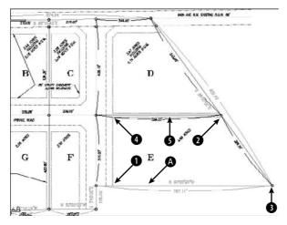
**4.** In the exercise on calculating area earlier in this chapter, you calculated a total area of 306975.04, in square inches. To calculate this area in square feet, type **quickcalc** →. In the Units Conversion section, choose Area from the Units Type drop-down list. In the Convert From drop-down list, choose Square Inches. In the Convert To drop-down list, choose Square Feet. In the Value to Convert text box, type **306975.04** →. AutoCAD calculates 2131.77111.
