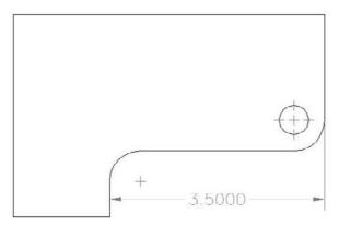
In the Dimension Break section, specify the break size. A dimension break is a gap in the dimension where it crosses an object. I discuss dimension breaks (the DIMBREAK command) in Chapter 14.
