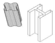
Note the I-beam in Figure 23.28. If you create an object by mirroring, stretching, and so on, you'll see extra tabulation lines at the separate segments in the polyline definition. If you want a clean look, you need to draw clean. You might need to use the original shape as a guide to draw a new polyline on top of the old one, and then erase the original.
