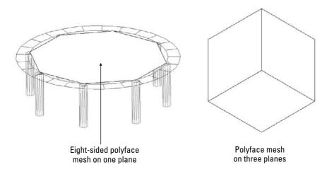
In order to easily draw a polyface mesh with PFACE, draw 2D or point objects as a guide for picking vertices. Then you can use object snaps to pick the vertices. Also, for polyface meshes on more than one plane, draw a diagram that numbers the vertices. This helps you to specify which vertices make up which face.
