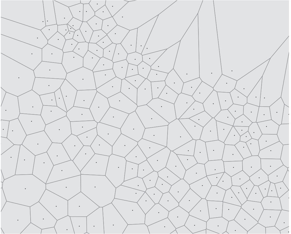
Fig. 4.3 Converting points to Thiessen polygons. An input layer of points is converted into an output polygon layer whose boundaries are equidistant from a pair of points. The Thiessen polygons and the points that created them are both shown.
