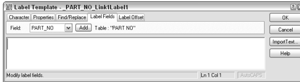
Figure 20-16: Use the Label Template dialog box to format and define label templates.
