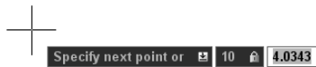
Figure 4-2: As you enter an X,Y coordinate, two boxes appear, one for each part of the coordinate.
