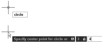
Figure 3-3: The Dynamic Input tooltip prompts you for input and then displays your input as you type.
