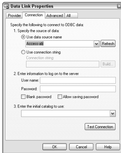
Figure 20-3: Use the Data Link Properties dialog box to configure your data source within AutoCAD.
