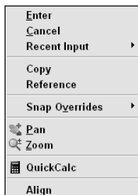
Figure 33-14: A custom command menu that appears when you right-click during the ROTATE command; the ALIGN command is at the bottom.
