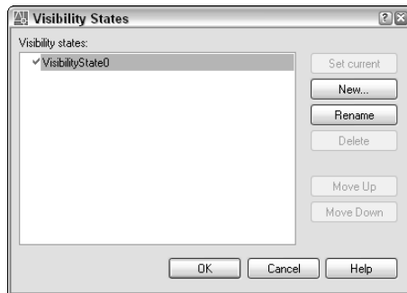
Figure 18-18: Use the Manage Visibility States dialog box to add and name visibility states.
