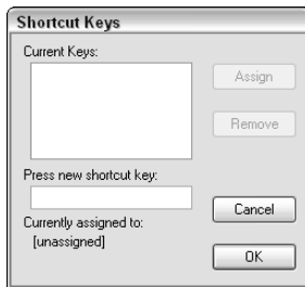
Figure 33-20: You assign shortcut keys to commands in the Shortcut Keys dialog box.
