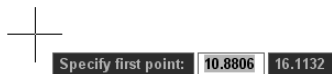
Figure 1-4: When you move the mouse around, the Dynamic Input bar follows the cursor, displaying the current coordinates.
