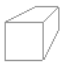
Figure 22-32: This model has a front clipping plane that hides the front of the model. Compare it to Figure 22-30.
