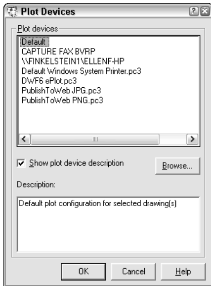
Figure 17-26: Use the Plot Devices dialog box to choose a plotter or printer for a drawing during batch plotting.
