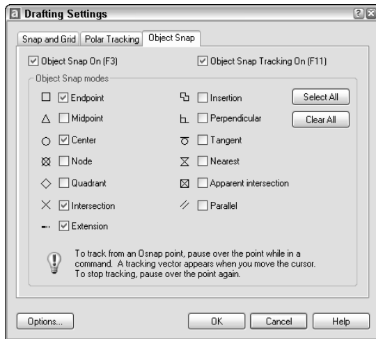
Figure 4-23: Use the Object Snap tab of the Drafting Settings dialog box to set running object snaps.
