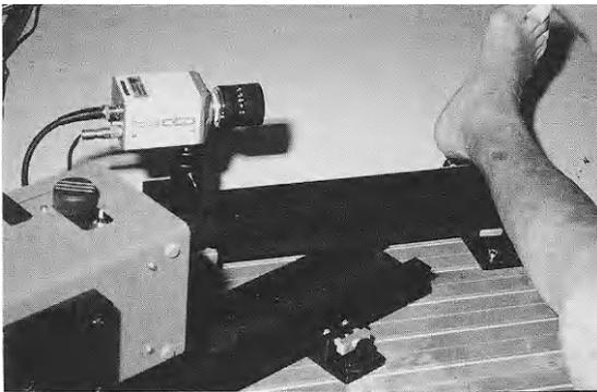
**Fig. 3.** Holon-View interferometry system. This special system is a prototype and was developed 3 years ago. The method has now been evaluated for study purposes
