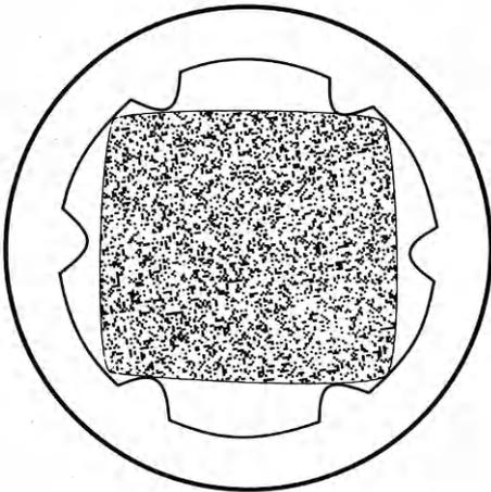
**Fig. 2.** Diagram representing cross section of the inner silicone rubber tube and cellulose sponge. Diameters of the tube are: outer diameter, 2.50 mm; inner diameter from furrow to furrow, 1.85 mm, from ridge to ridge, 1.58 mm. The sponge is 1.3 × 1.3 × 20 mm in size
