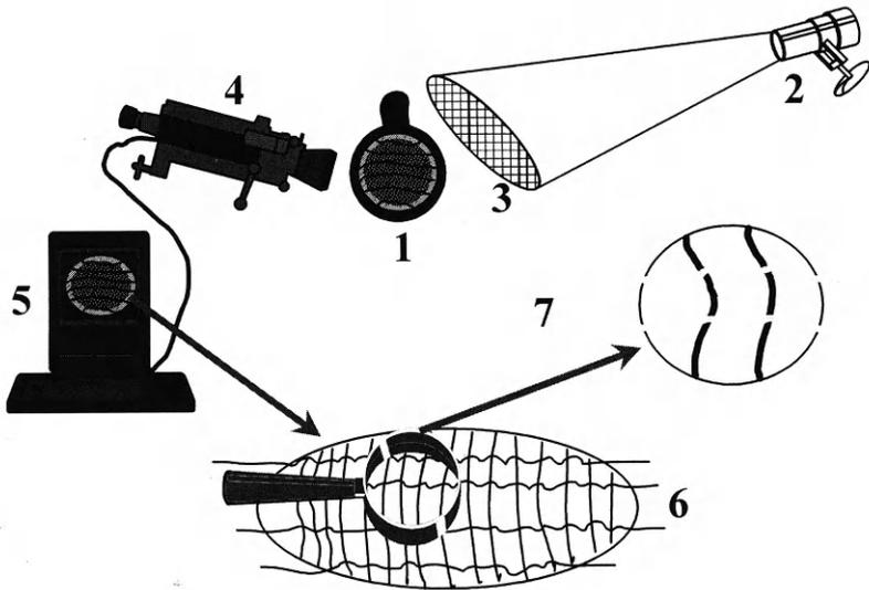
**Fig. 4.** Holon-View, technical principle. The examination object (1) is illuminated by a projector (2), projecting a grid line pattern onto the object (3). The object is recorded by a video camera (4) and transferred to the computer for further processing (5). By using the gray code sequence technique, each image point is converted into intensity and height values (6,7)
