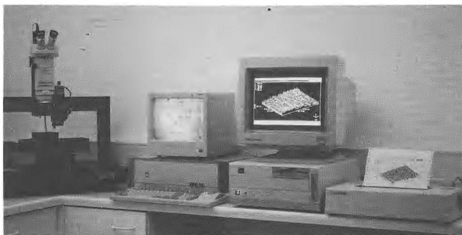
**Fig. 9.** Laser profilometry unit UBC 14 working place with profilometer, video microscope, computer unit, and printer
