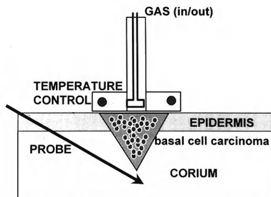
Fig. 1. Functional diagram of a closed cryosystem. The cryoprocess causes a triangular defect
