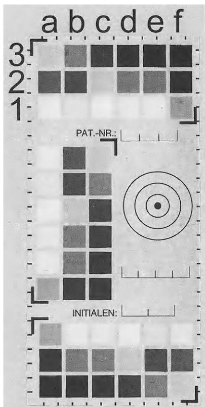
**Fig. 1.** Reference card used for color correction and distance calibration
