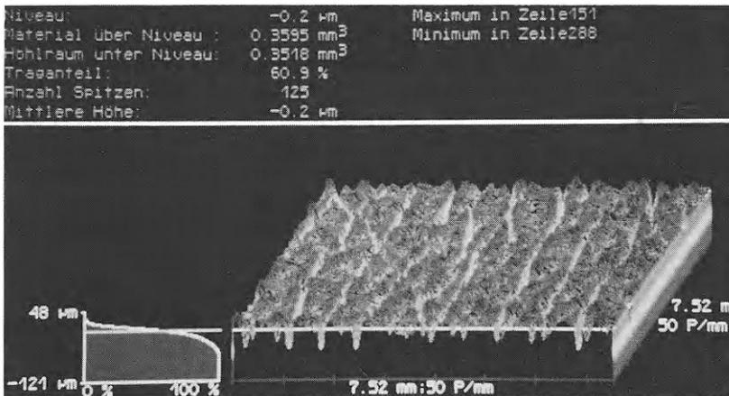
**Fig. 11.** Laser profilometry image. Volume determination in relation to freely chosen height lines can easily be performed. The architecture of skin lines can be recognized in the image. The volume determination is very useful to evaluate the treatment of scars. We combine the interferometry (large scars) with laser profilometry (small scars)
