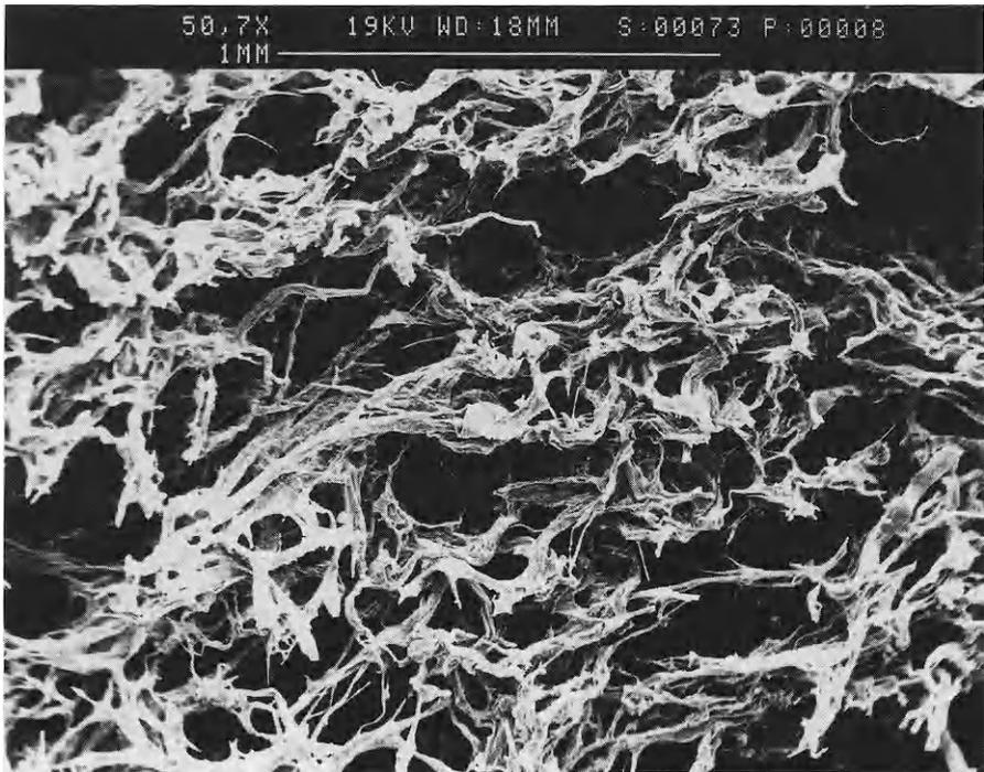
**Fig. 3.** SEM picture of the Cellstick cellulose sponge. Note 1 mm scale at the upper margin of the picture
