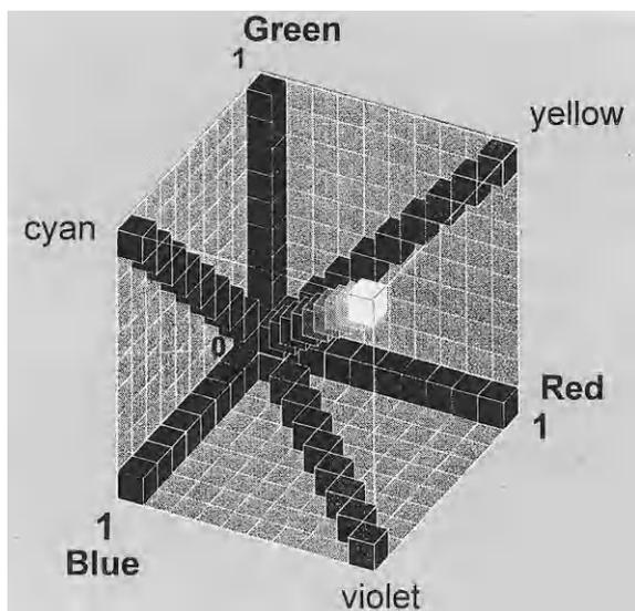
**Fig. 3.** The RGB color coding system can be represented as a cube. Every color is described by three cartesian coordinates (R,G,B), which describe its red, green, and blue intensity. Their intensity varies between 0 and 1. The corners of the cube are red (1,0,0), green (0,1,0), blue (0,0,1), yellow (1,1,0), cyan (0,1,1), violet (1,0,1), black (0,0,0), and white (1,1,1). Shades of gray are located on the black–white diagonal
