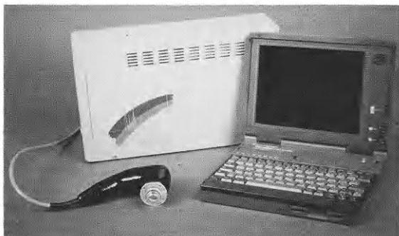
**Fig. 2.** DUB 20S 20-MHz sonography unit. Both commercial available system (DUB 20 and Dermascan C) are comparable and do not differ very much in the technical possibilities for routine diagnostics
