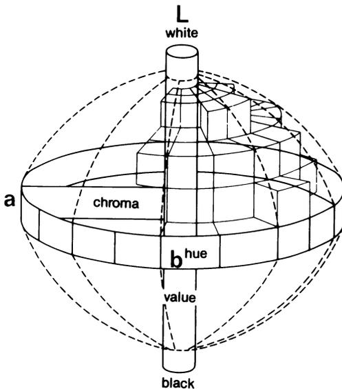
**Fig. 2.** The Lab color representation system forms a three-dimensional ovaloid, where all possible colors are included. L, lightness factor; a, red–green axis; b, blue–yellow axis. By moving in a radial direction, the chroma (saturation) of the color changes; by moving circularly, its hue changes
