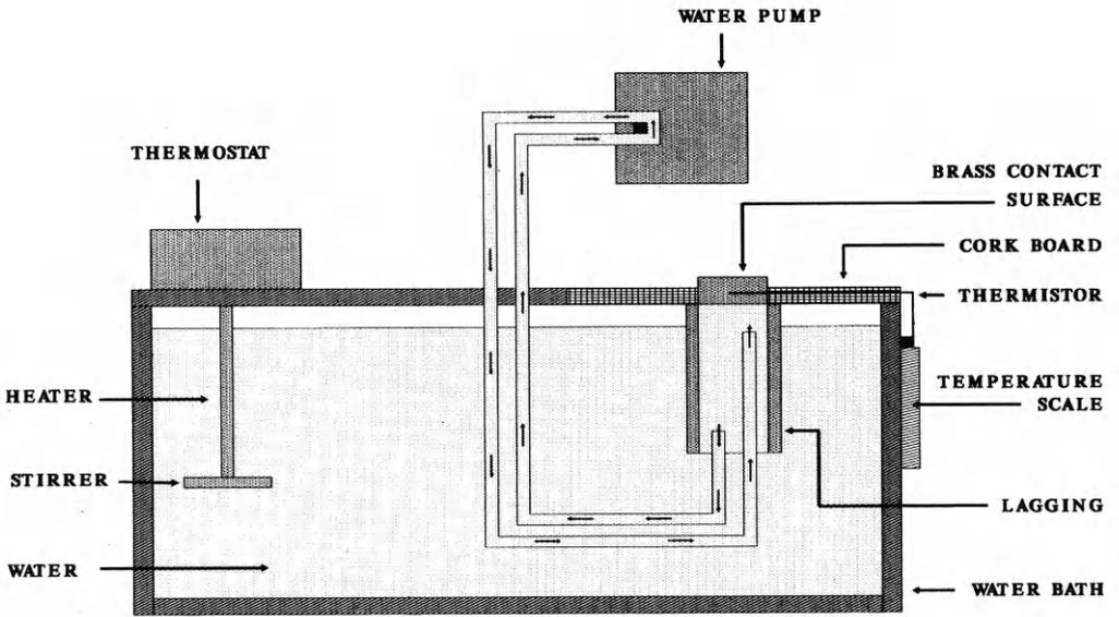
Fig. 1. Apparatus for the rat thermal injury model
