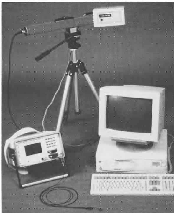
**Fig. 13.** Laser Doppler imaging system (LDI). This Swedish system is commercially available
