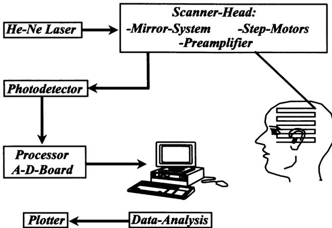
Fig. 1. A laser Doppler scanner
