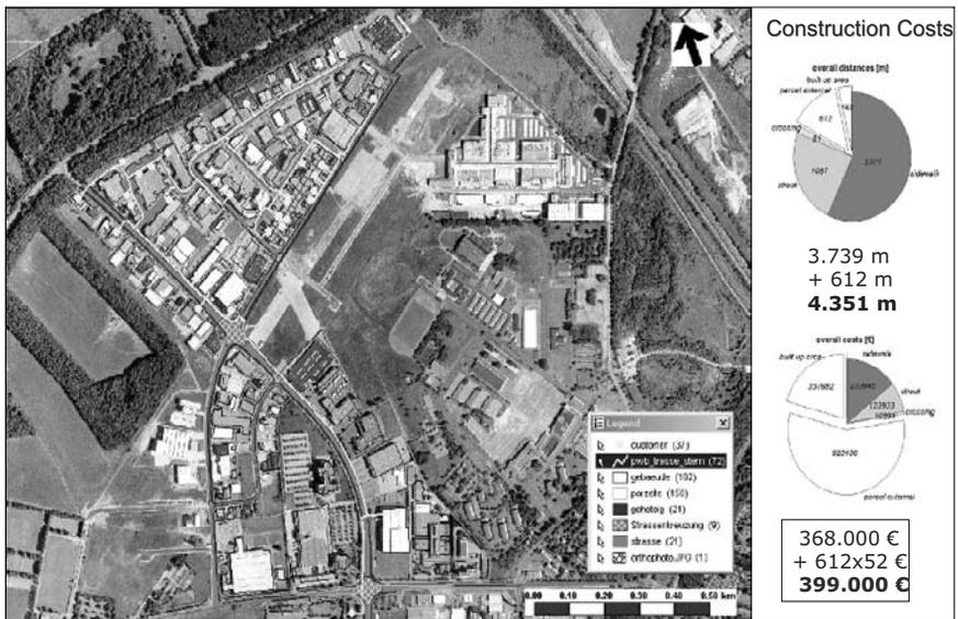
**Fig. 5.** Visualization of a cost optimized fibre optic network design together with expected construction costs for one specific scenario. (Benchmark project implemented for industry partner NetCologne in Köln-Ossendorf, Germany).
