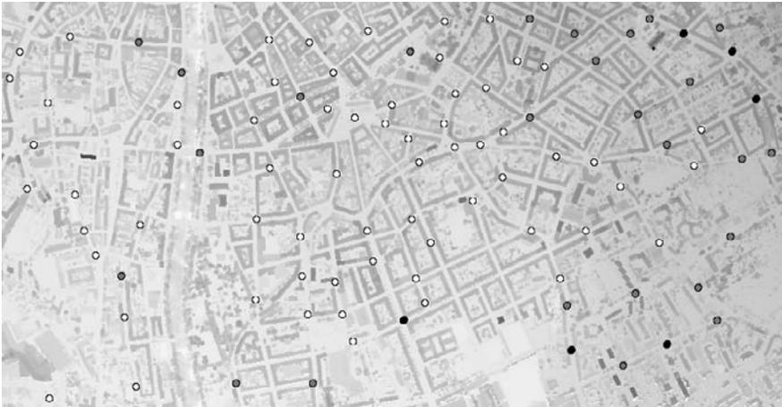
**Fig. 5:** Manually selected points which are used for calculating the height difference. White points show the minimum error.
