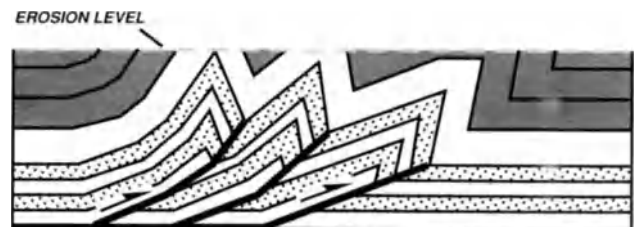
Figure 3. Blind thrust system formed by a buried imbricate fan in which the overlying strata are shortened by folding.
