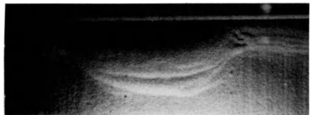
Figure 12. Photo of a sand lobe formed in front of the notched indenter sketched in Figure 8. This photo is taken looking vertically down on the surface, and movement is from the top to the bottom of the photo. The lobe, which is 15 cm-long measured parallel to the indenter face, forms where the sand being pushed by the indenter is thicker. Note that the spacing of faults depends on wedge width.
