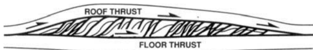
Figure 31. Smooth roof duplex where the roof thrust varies smoothly without folding by the underlying link thrusts (adapted after McClay & Insley 1986).
