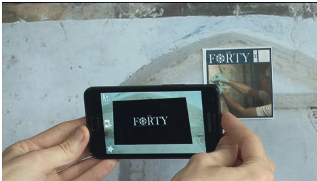
Fig. 15.1 The Aurasma application displaying a film clip on a smart phone, the playing of which has been triggered by “recognizing” the paper glyphs attached to the poster
