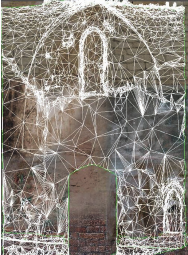
Fig. 16.1 Textured mesh converted from point cloud data
