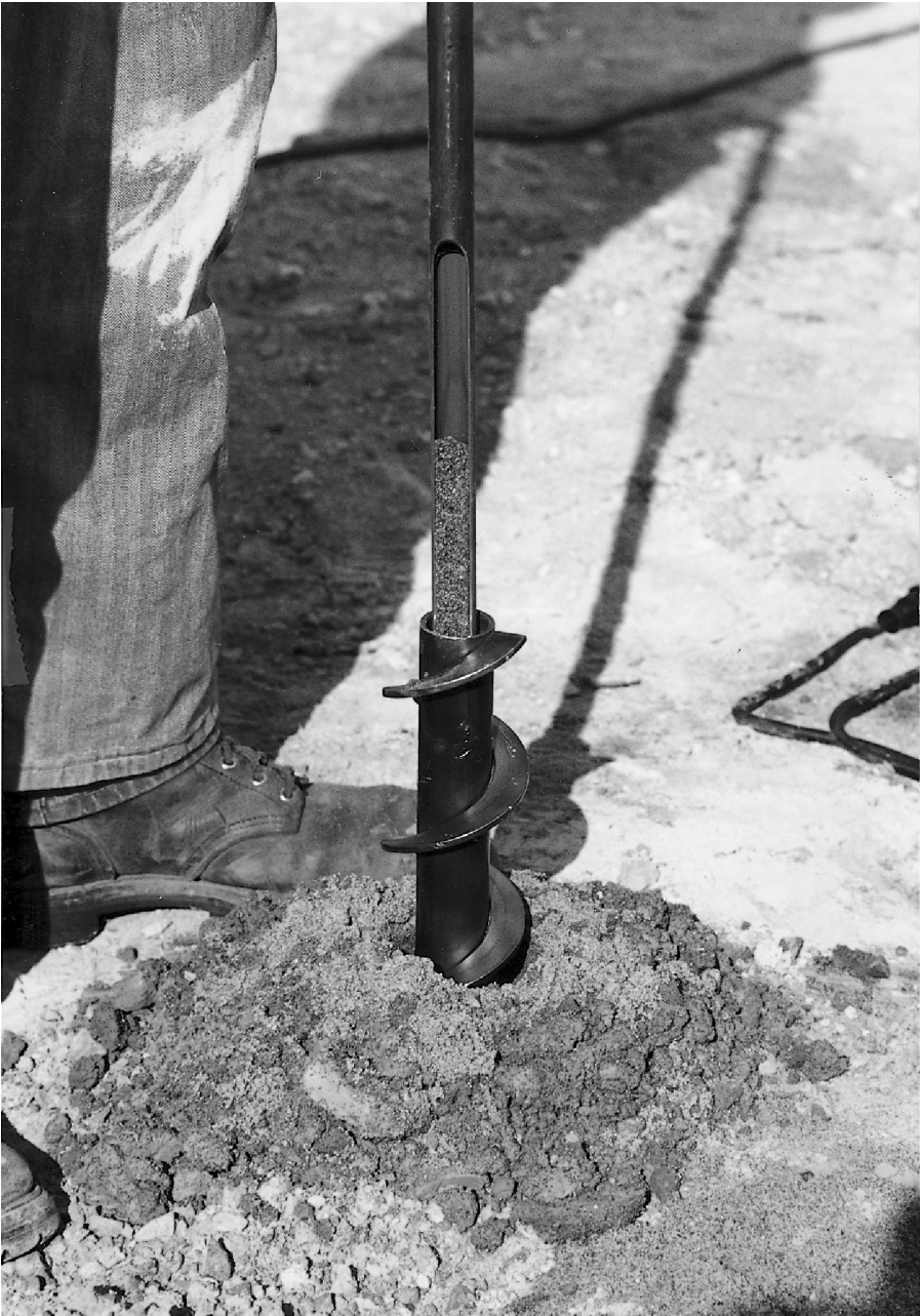
Figure 8.6. A handheld auger drilling system. (Courtesy of Forestry Suppliers, Inc. http://www.forestry-suppliers.com ).
