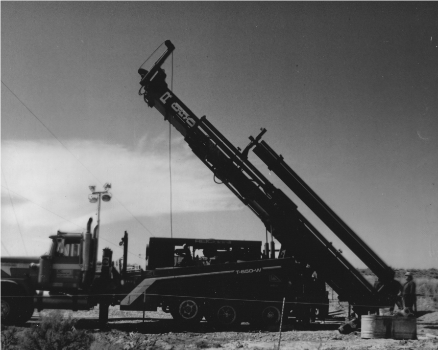
Figure 8.5. A direct rotary drill rig being used to drill a diagonal well (U.S. DOE-INEL photograph).
