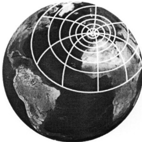
Figure 6.14. Sketch of a variable-resolution grid in a general circulation model such as the French ARPEGE model, where sharper resolution is obtained in a region of interest at the expense of lower resolution elsewhere.
