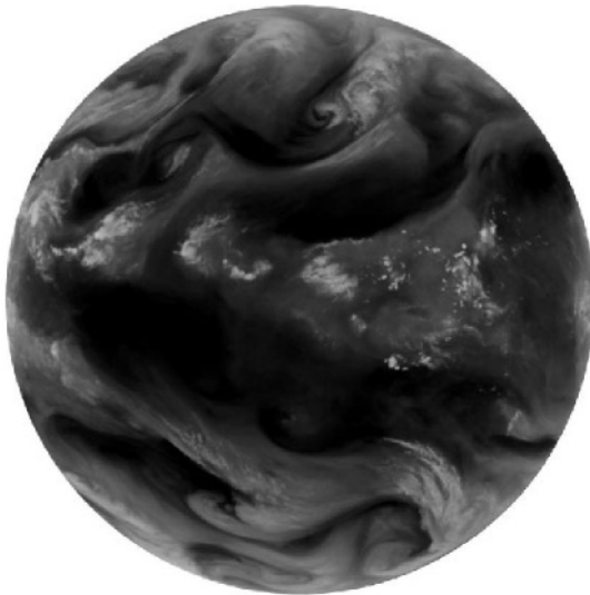
Figure 5.21. A view with the Meteosat water vapor sensor. Bright regions denote high water vapor content, dark regions are associated with very dry air masses. The satellite does not “see” the Earth’s surface as neither oceans nor land emit in the water-vapor bands (Courtesy: European Space Agency).
