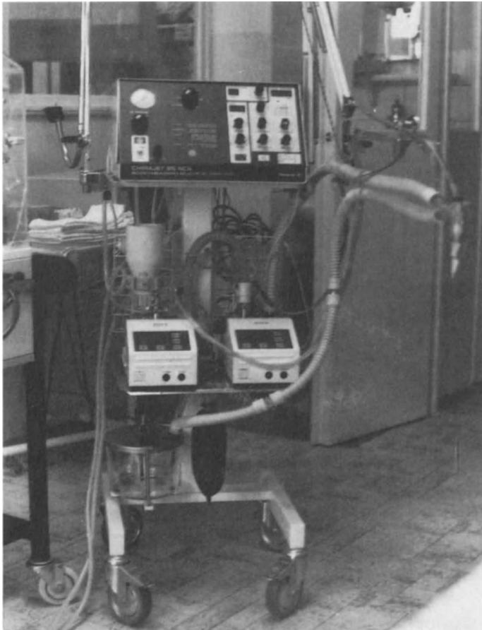
Figure 6. Czechoslovak high frequency jet ventilator – clinical type with low-pressure and high-pressure humidifiers
