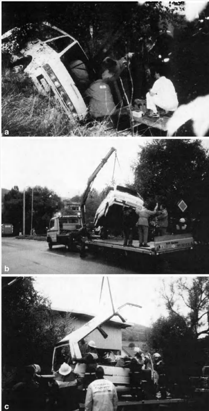
Fig. 4a–c. Bringing a car to a stable condition before extrication
