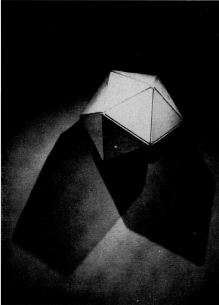
FIG. 27. A model of an icosahedron shadowed by two light sources and oriented so that an apex of the hexagonal contour points directly to each light source. This throws two shadows, one is four-sided and pointed, and the other is five-sided with a blunt end. (From Williams and Smith, 1958.)
