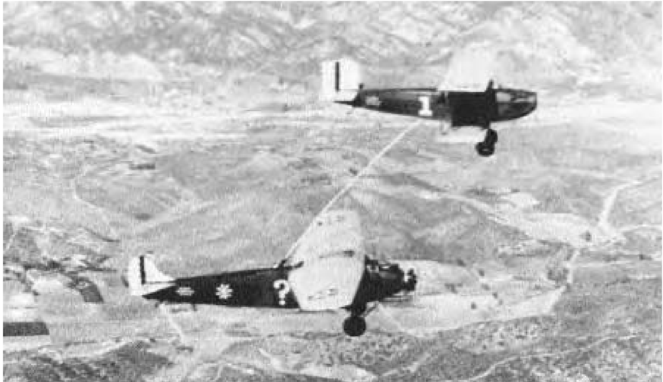
The flight of the Question Mark demonstrated that aerial refueling would be important in the future, but it did not come into extensive use until well after World War II. (U.S. Air Force)
