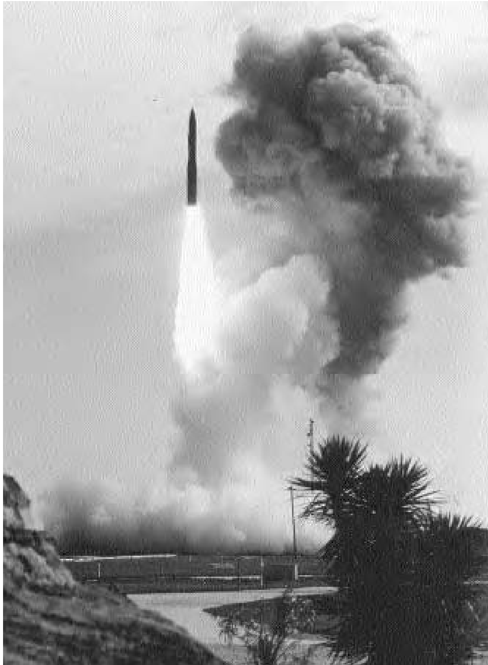
Solid rocket fuel made the Minuteman missile much easier to service and to launch. (U.S. Air Force)
