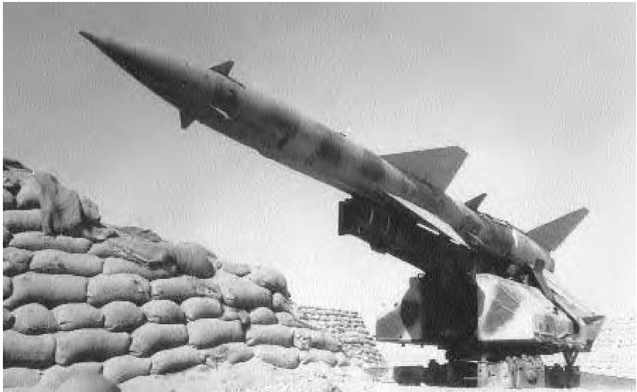
A direct descendant of the German Wasserfall missile, the Soviet Union's SA-2 Guideline was one of the most important surface-to-air missiles ever built. (Lon Nordeen)
