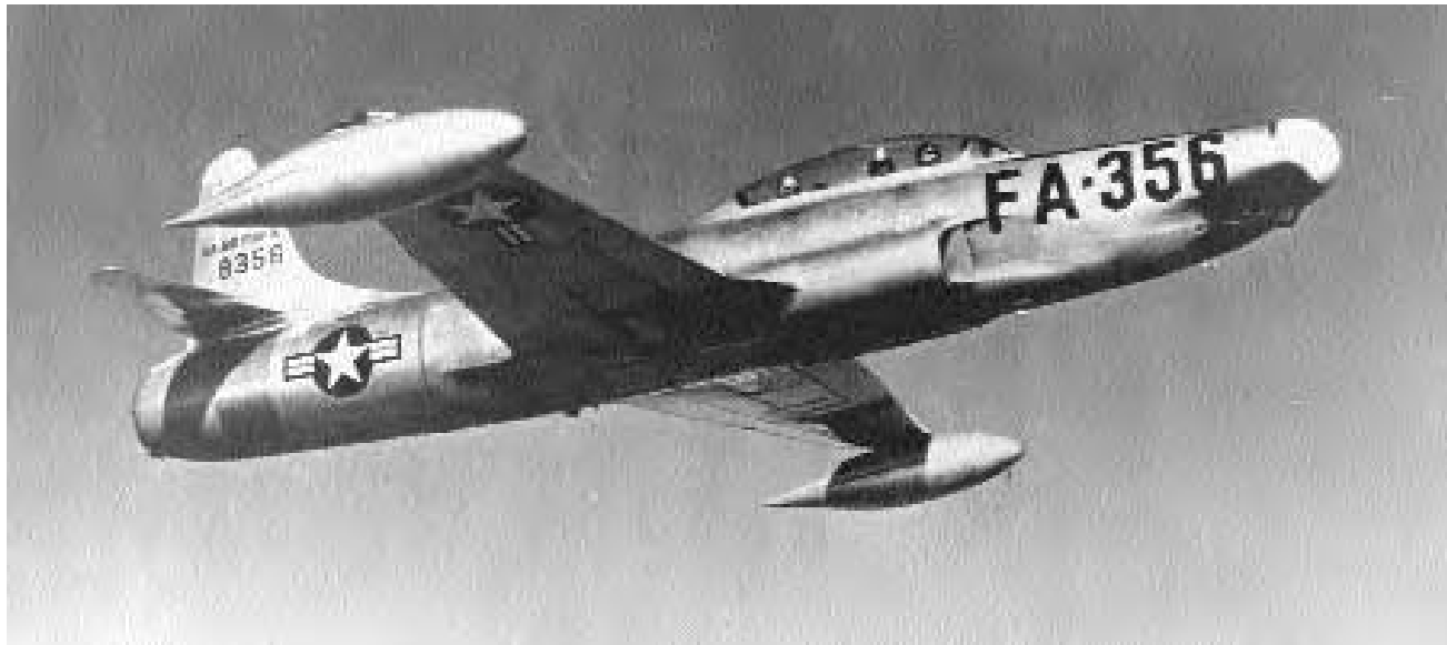
The interception of bomber aircraft under all weather conditions was a very difficult proposition, and the Lockheed F-94 was derived from the basic T-33 as an interim measure. (Walter J. Boyne)
