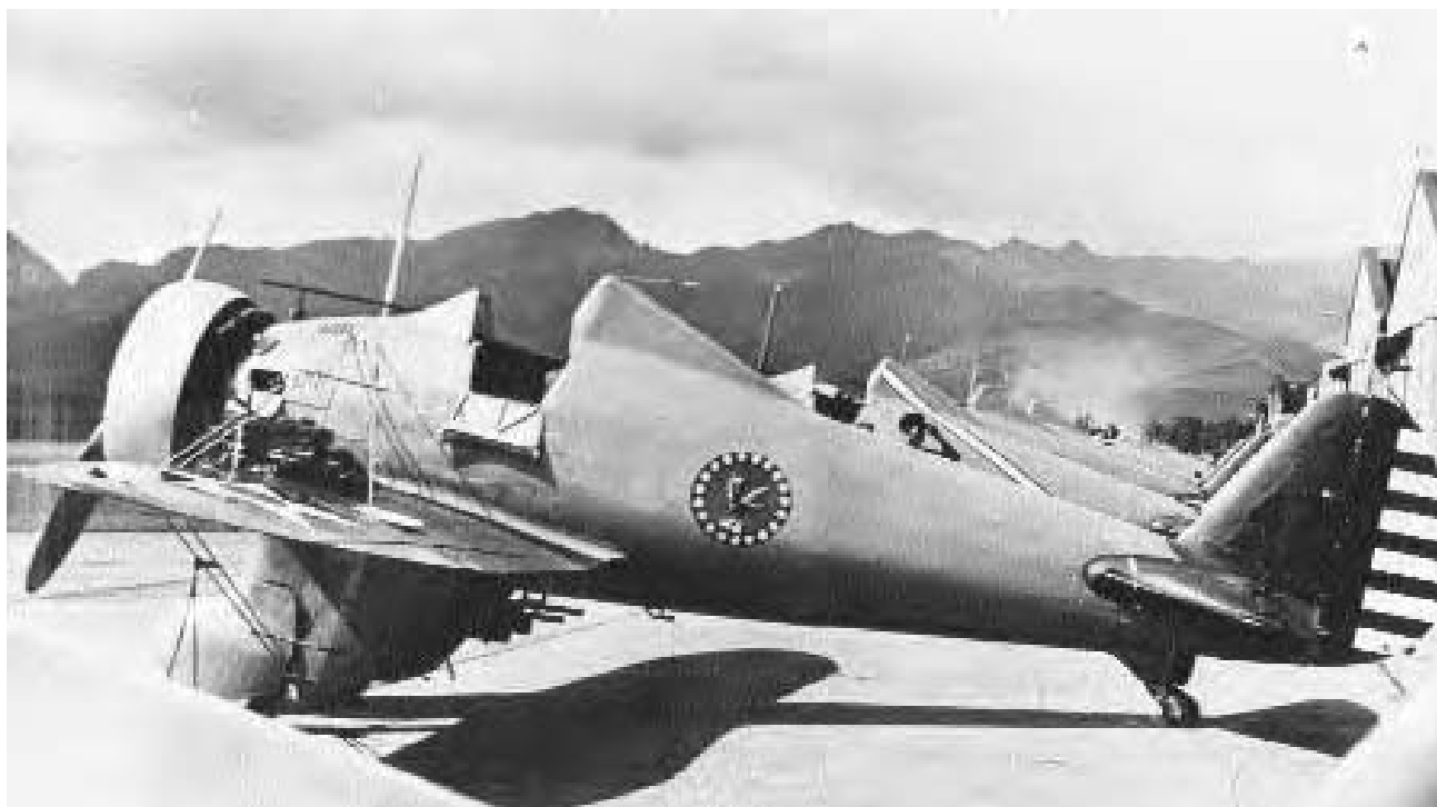
The Boeing P-26 "Peashooter" was a transitional aircraft. The all-metal monoplane retained the open cockpit and fixed gear of its biplane predecessors. (U.S. Air Force)
