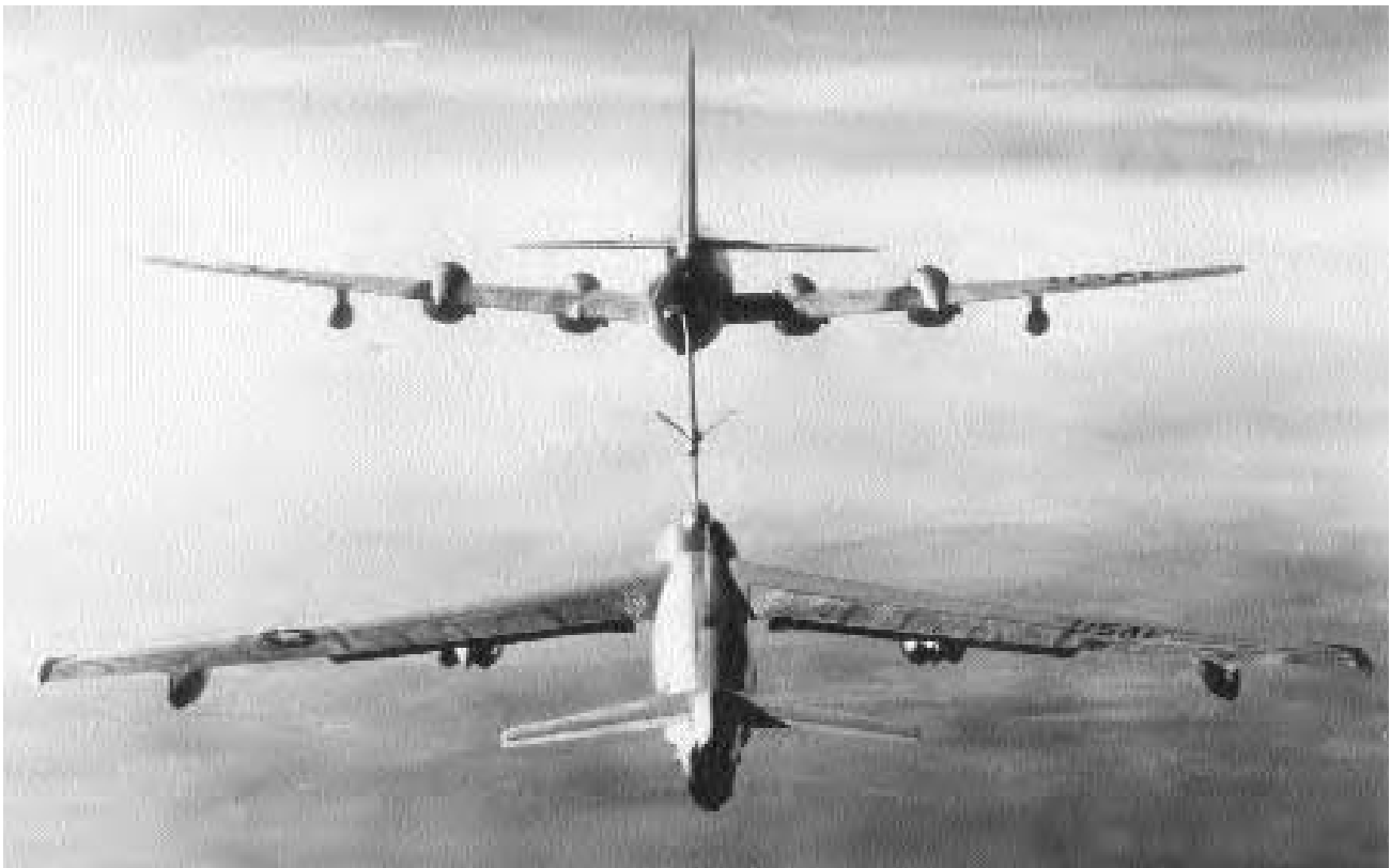
Refueling a six-jet Boeing B-47 from a six-engine (four-piston, two-jet) Boeing KC-97 was no easy task, for the tanker had to fly at top speed, sometimes in a descent. As you can tell from the nose-up attitude of the B-47, it is flying as slow as it can and still not stalling. (U.S. Air Force)
