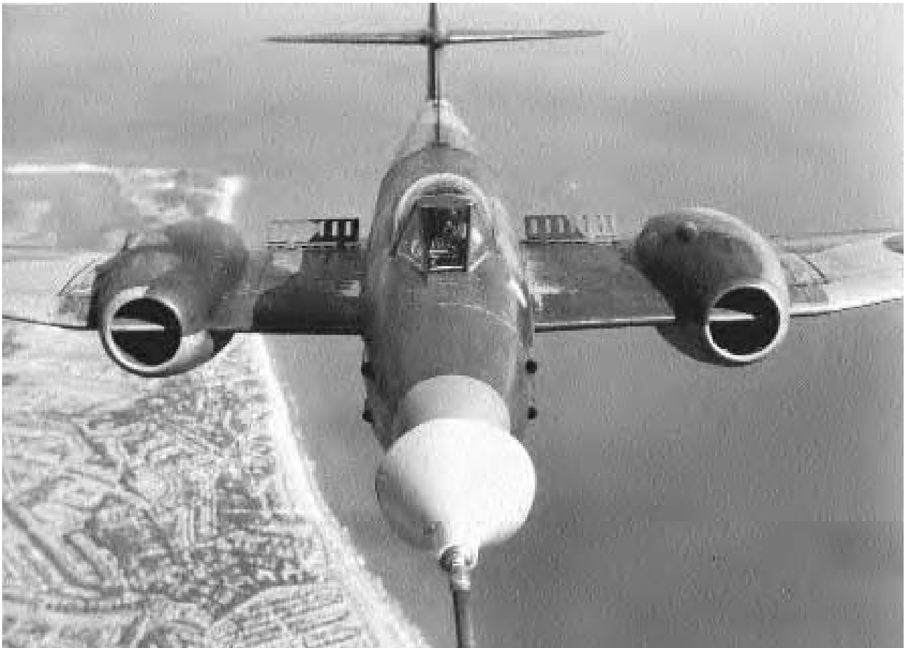
The Gloster Meteor became a work horse for the RAF, serving many test purposes, including inflight refueling. (Walter J. Boyne)
