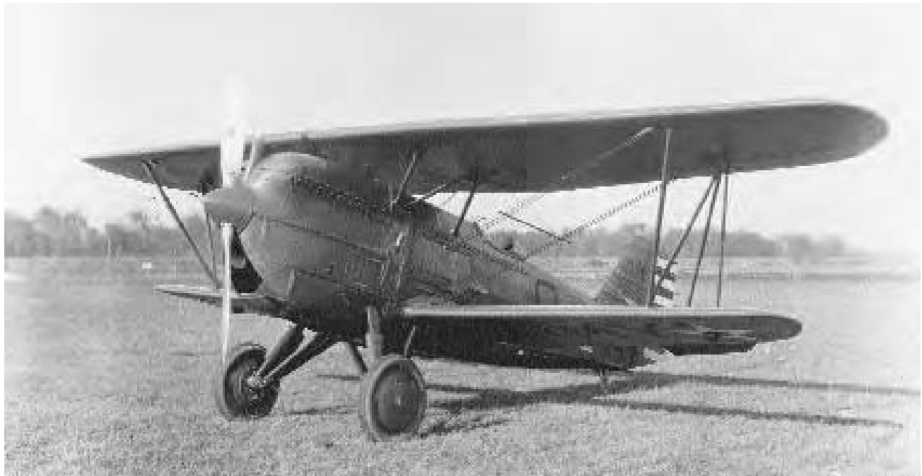
The Curtiss P-6 was modified over the years but retained the same basic formula of World War I fighters as an open cockpit biplane with fixed landing gear and fixed propeller. (U.S. Air Force)
