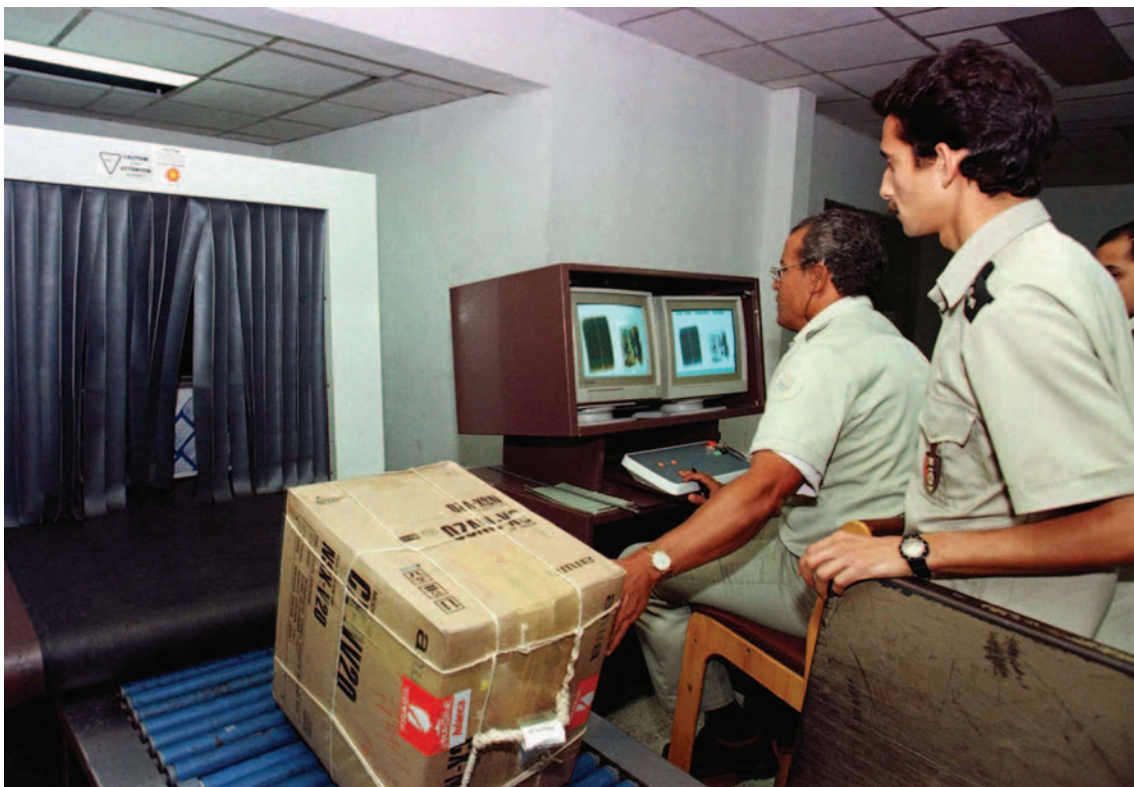
Security personnel use equipment that features californium-252 to inspect luggage. AP IMAGES.
