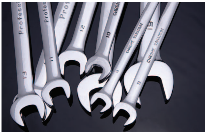
Wrenches made with a vanadium steel alloy. IMAGE COPYRIGHT 2009, STEVE COLLENDER. USED UNDER LICENSE FROM SHUTTERSTOCK.COM.
