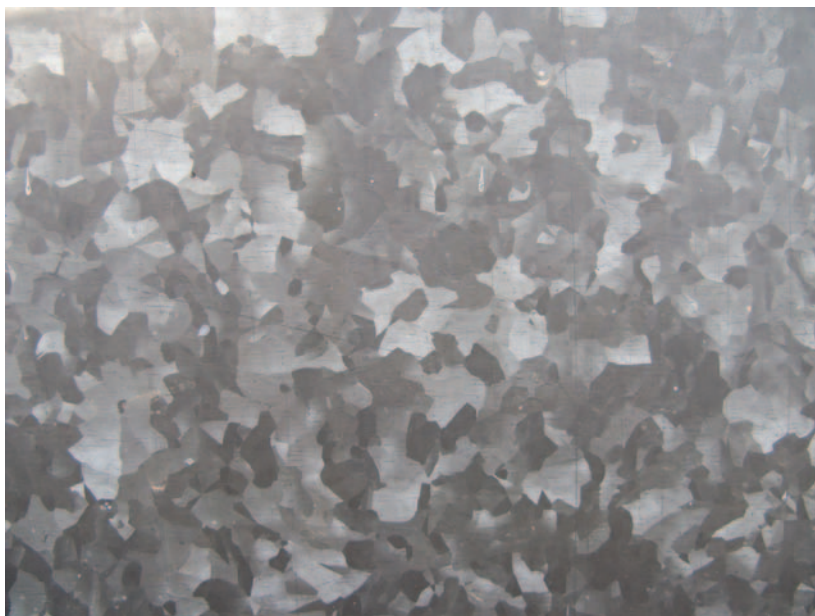
Zinc is used to galvanize other metals, particularly iron and steel. A zinc-plated metal surface is shown here. IMAGE COPYRIGHT 2009, ZTS. USED UNDER LICENSE FROM SHUTTERSTOCK.COM.
