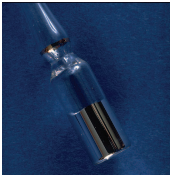
Sample of rubidium stored in hydrogen. © RUSS LAPPA/SCIENCE SOURCE, NATIONAL AUDUBON SOCIETY COLLECTION/PHOTO RESEARCHERS, INC.
