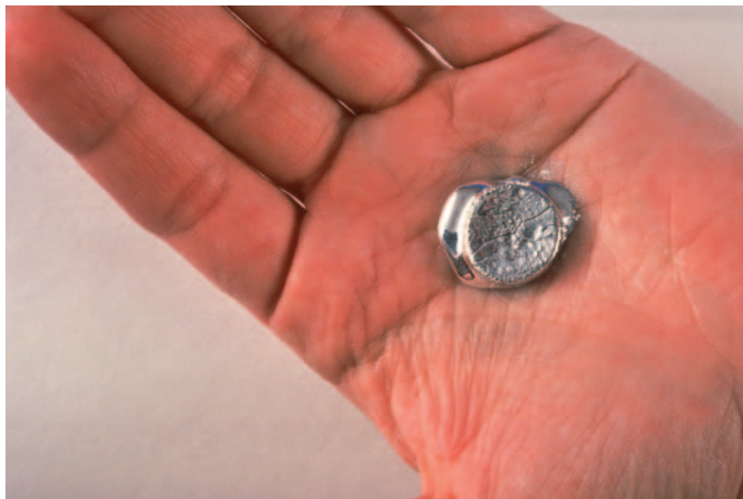
Gallium melts when held in one's hand. © RUSS LAPPA/SCIENCE SOURCE, NATIONAL AUDUBON SOCIETY COLLECTION/PHOTO RESEARCHERS, INC.
