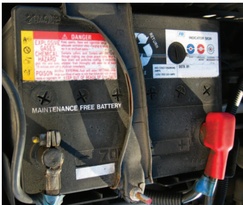
Common lead storage batteries used in cars and trucks contain alloys of arsenic. IMAGE COPYRIGHT 2009, ALBERT LOZANO. USED UNDER LICENSE FROM SHUTTERSTOCK.COM.
