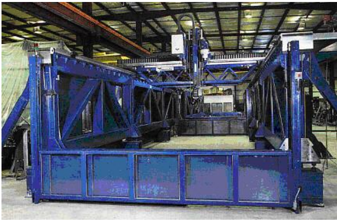
Fig. 10.25. Large 5-axis gantry for laser maskant scriber driven by Anorad's LSMs. Photo courtesy of G. Hagiz [76].
