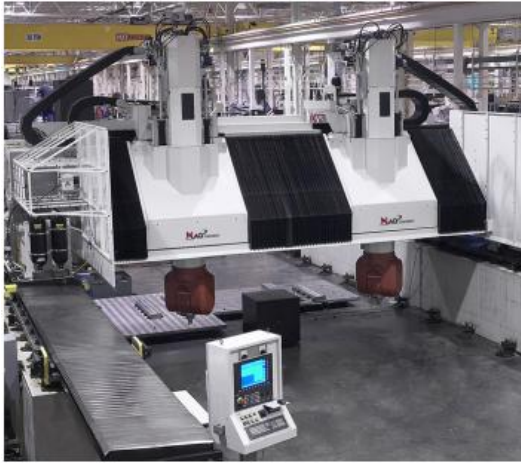
Fig. 10.20. HyperMach TM vertical profiler with PM LSMs in the x and y axes. Photo courtesy of MAG, Hebron, KY, USA.
