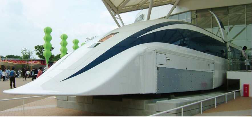
Fig. 8.19 Double-cusp-shaped head car (facing Koufuu) of the MLX01 Maglev Train at Expo 2005, Aichi Prefecture, Japan. Courtesy of Central Japan Railway Company and Railway Technical Research Institute, Tokyo, Japan.
