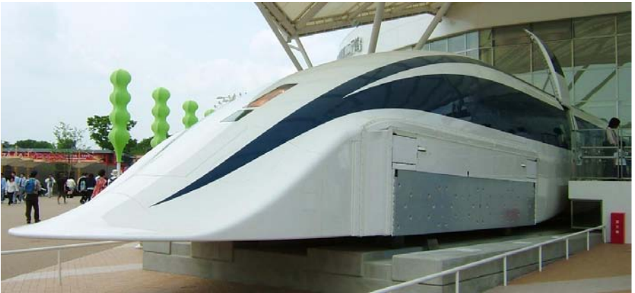
Fig. 8.19. (see color insert.) Double-cusp-shaped head car (facing Koufu) of the MLX01 Maglev Train at Expo 2005, Aichi Prefecture, Japan. Courtesy of Central Japan Railway Company and Railway Technical Research Institute, Tokyo, Japan.
