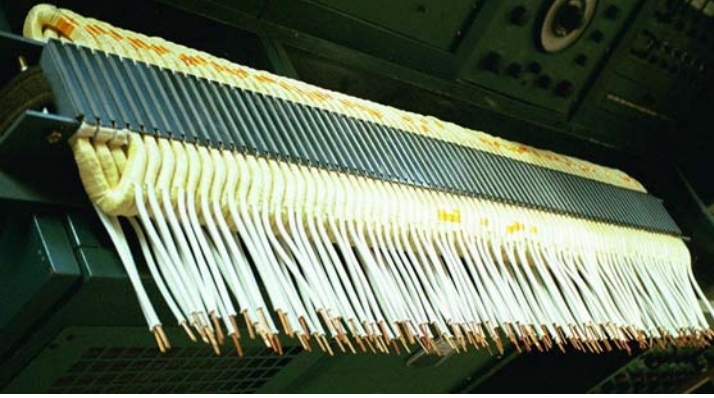
Fig. 2.22. Double-layer winding wound with rectangular cross section wires of a large PM LSM. Photo courtesy of Dr. S. Kuznetsov, Power Superconductor Applications Corp., Pittsburgh, PA, USA.
