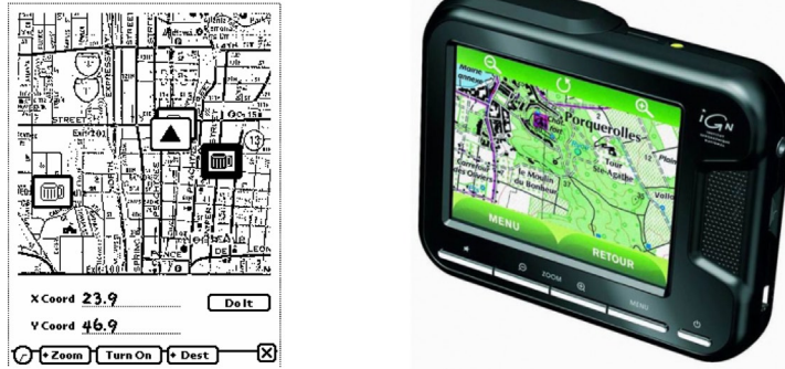
FIGURE 8.7: Shown left is a screenshot of the Cyberguide system from 1996. Shown right is the Evadeos device designed and sold by France’s National Geographical Institute. The Evadeos features GPS, a database with 1.7 million points of interest and a facility to add new content via radio or flash memory.
