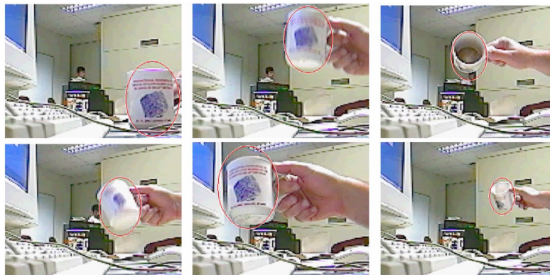
FIGURE 6.5: Samples images from a real-time vision-based system that can track an object after it is manually identified on the video [28]. © 2003 IEEE.
