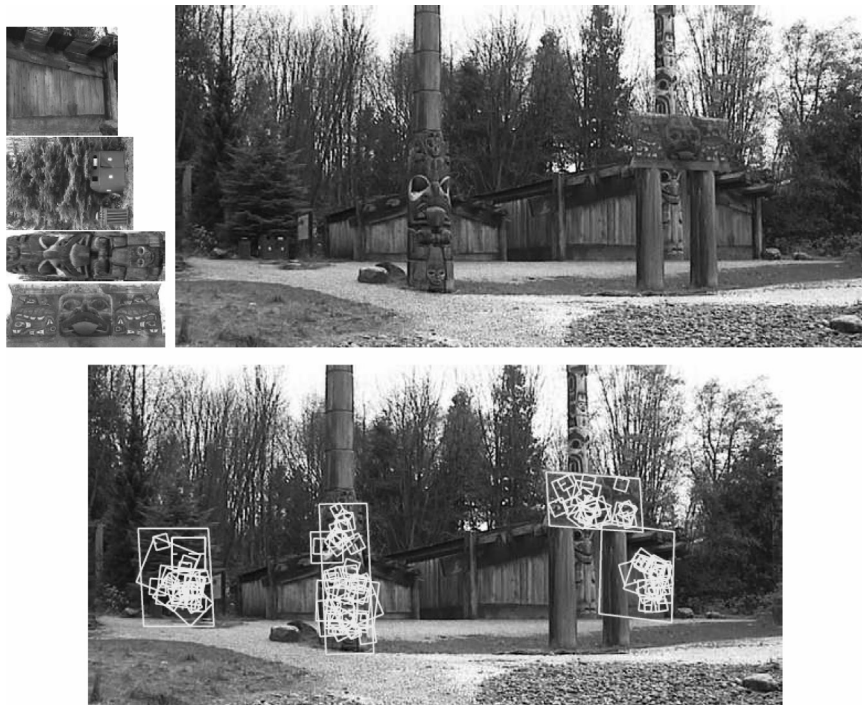
FIGURE 6.2: An example of SIFT feature recognition. Images of previously learned landmarks are shown upper left. The lower large image shows the scale and viewpoint invariant recognition of these landmarks in the upper large image [104]. © 1999 IEEE.
