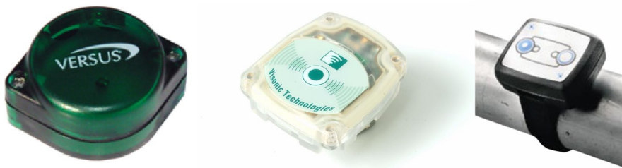
FIGURE 8.3: Three asset tags capable of providing real-time location information. Shown left is an infrared tag made by Versus, shown middle is an infrared tag made by Visonic, and shown right is a 802.11 beacon tag made by Ekahau.
