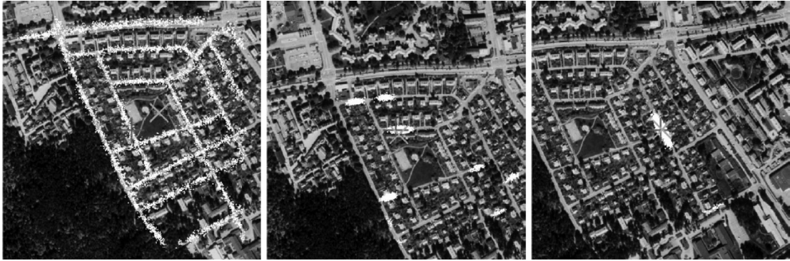
FIGURE 7.7: These three images show a particle filter tracking the location of a car using turn information alone. With each successive turn the system become more confident of the street the car is on. [62]. © 2002 IEEE.
