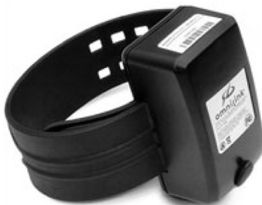
FIGURE 8.5: OmniLink’s “Offender Tracking Technology” bracelet uses GPS and cell-tower location for indoor and outdoor location estimation. The ankle bracelet is shown left, and a snippet of their profile creation tool is shown right.
