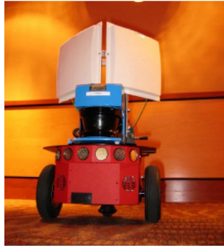
FIGURE 6.11: The two white RFID readers can guide this robot with 2 m accuracy without the assistance of the laser range finder [64]. © 2004 IEEE.
