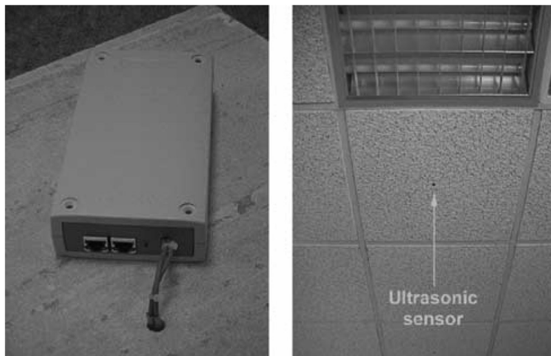
FIGURE 3.8: Ultrasound receiver unit for Active Bats. Shown sitting on ceiling tile (left) and shown when installed (right) with only receive sensor exposed [66]. © 2002, ACM, Inc. Reprinted by permission.
