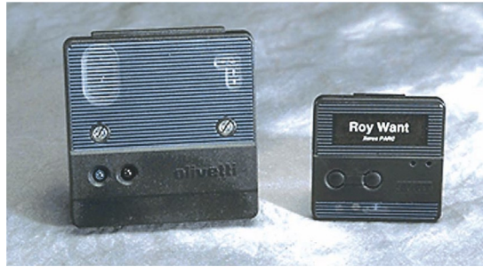
FIGURE 3.1: An Olivetti Active Badge (right) and the sensor base station (left) used to watch for badges [68].
