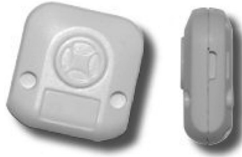
FIGURE 6.12: A UbiSense compact ultrawide-band tag (25 g).
