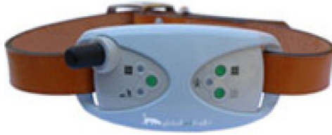
FIGURE 8.6: The 200-g Global Pet Finder collar uses GPS to locate and the cellular network to alert owners of a pet’s location when it has wandered.
