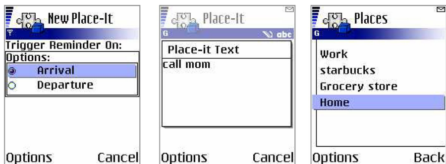
FIGURE 8.10: This sequence of phone screens illustrate how users of the Place-Its system author new location-based reminders, in this case, to "Call mom when I get home."
