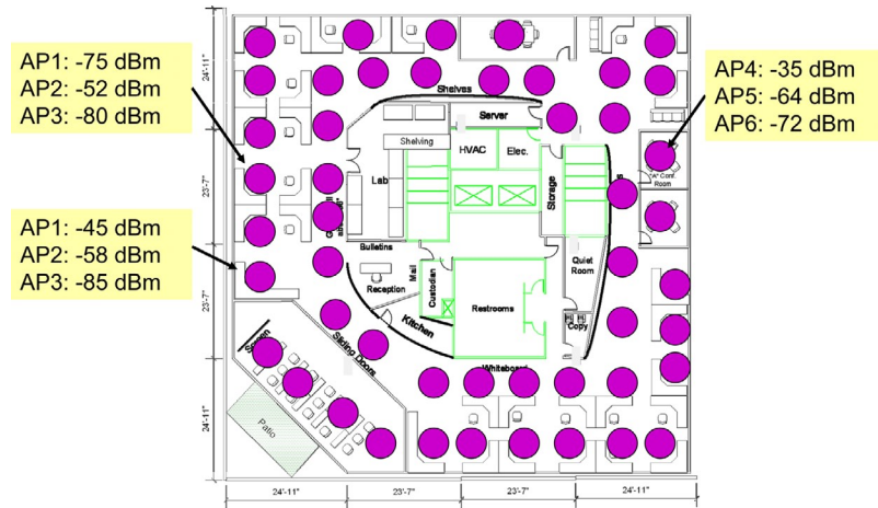
FIGURE 4.3: This map of an indoor office environment shows a reasonable set of locations in which to collect scans for a radio map. The three sample scans show that AP signal strength will vary across location and may potentially contain nonoverlapping sets of APs.
