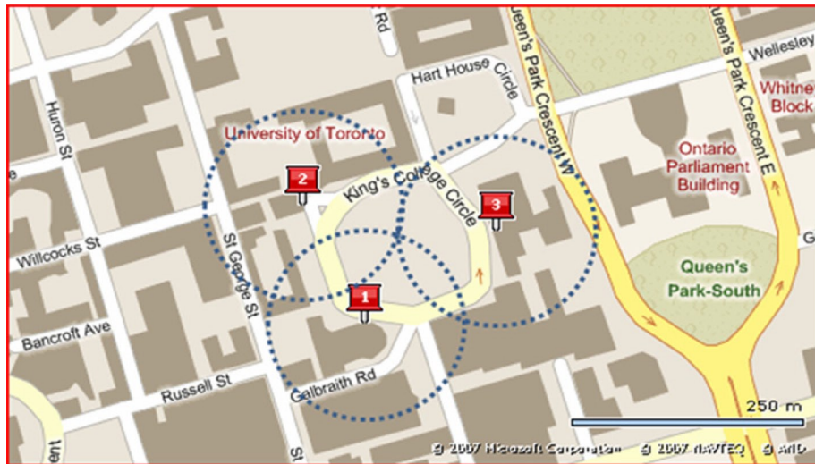
FIGURE 4.9: Predicted client location based on observation of three 802.11 APs.
