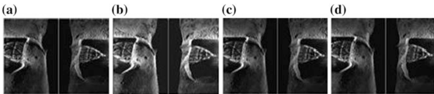
Fig. 5 a Original ‘hurricane gate’ (image courtesy of M/s Edgetech), b enhanced image using PSO, c median filter, and d adaptive Wiener filter
