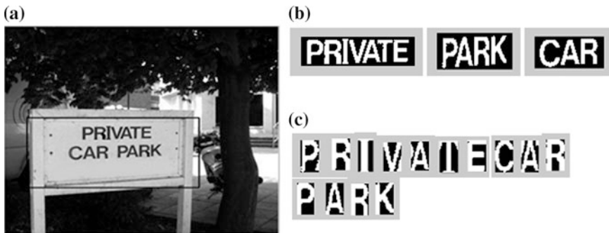
Fig. 1 Results of our proposed methodology. a Scene image, b representing the extracted region, and c segmented text extracted using our proposed methodology
