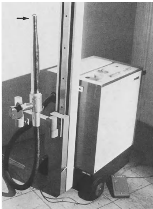
Fig. 10. Philips unit RT 50 used in intracavitary irradiation of rectal cancer. The X-ray tube is shown by the arrow
