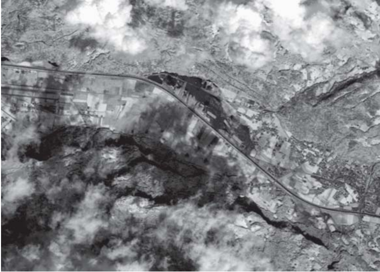
Fig. 2 A section of the SPOT5 near-infrared band showing the spectral similarity of flooded areas and shadows
