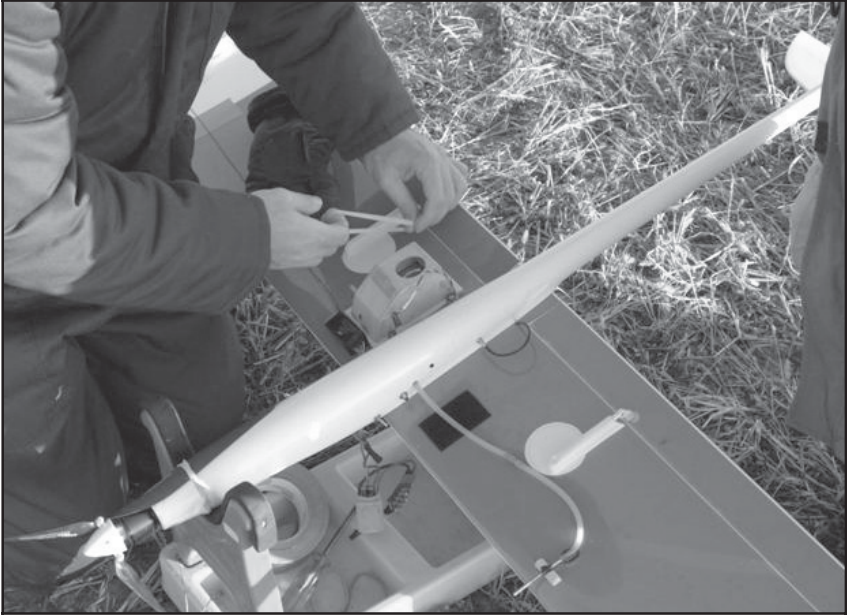
Fig. 3 Detail of the camera mounting system
