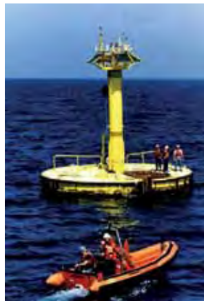
Figure 3.8 An automated weather buoy. This one is 10 m across – note the size of the scientists on board. (Photo: NOAA.)
