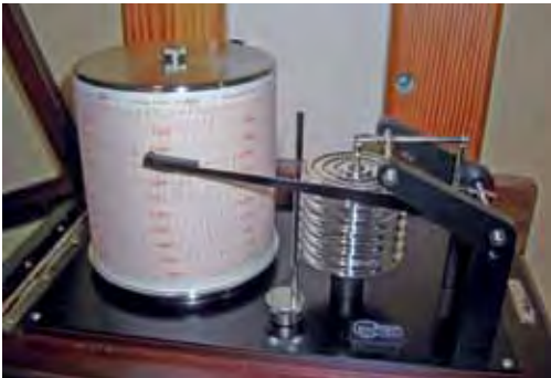
Figure 3.4 This barograph measures pressure using an aneroid capsule, which is linked mechanically to an arm with a pen on the end. The drum on the left rotates slowly, allowing the pen to trace out changes in pressure on the chart. (Photo: Department of Meteorology.)
