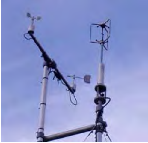
Figure 3.3 Instruments for measuring wind: a traditional cup anemometer (left), a wind vane (centre) and a sonic anemometer (right). The sonic anemometer measures wind speed by emitting pulses of sound waves and timing their journey from transmitter to receiver. (Photo: Department of Meteorology.)
