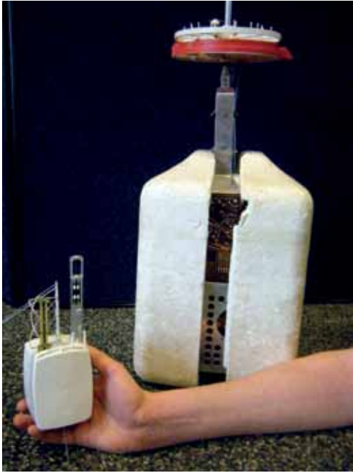
Figure 4.1 Modern radiosondes now fit in the palm of a meteorologist's hand – much more compact than earlier designs. The large radiosonde at the back dates from the 1970s. (Photo: Department of Meteorology.)
