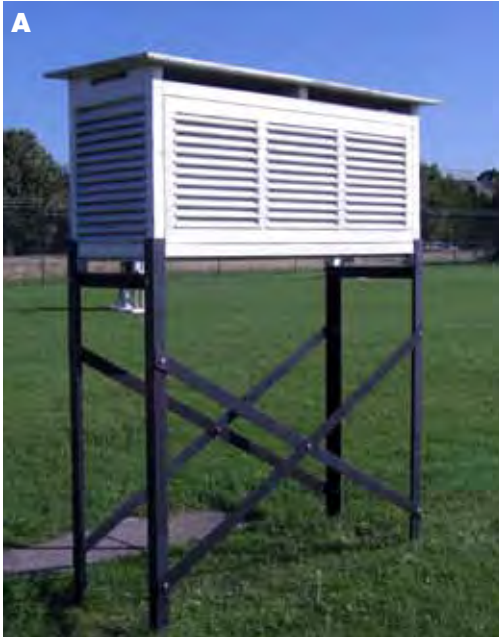
Figure 3.2 (A) A modern Stevenson screen. (B) The standard arrangement of thermometers inside consists of dry-bulb and wet-bulb thermometers (mounted vertically to the left and right respectively) and maximum and minimum thermometers (mounted horizontally, top and bottom). (Photos: Department of Meteorology.)
