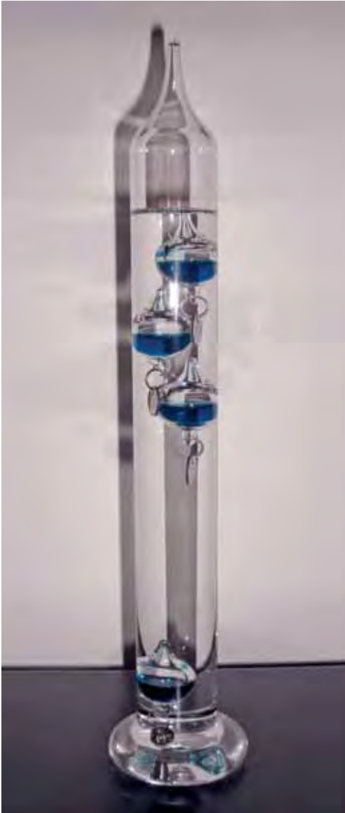
Figure 2.2 A Galileo thermometer. Each glass sphere floats at a different temperature, indicated by the metal tag on the bottom. The temperature here is 21°C. (Photo: Jon Shonk.)
