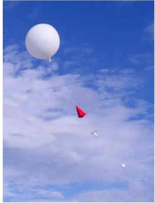
Figure 4.2 A radiosonde launch. The assembly consists of a radiosonde (the small white box at the bottom), a parachute (the red piece of plastic) and a helium balloon, which usually measures about 2 m across at launch. (Photo: Department of Meteorology.)
